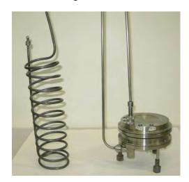
Figure 1 – Pre-saturator (L) and saturator (R)
