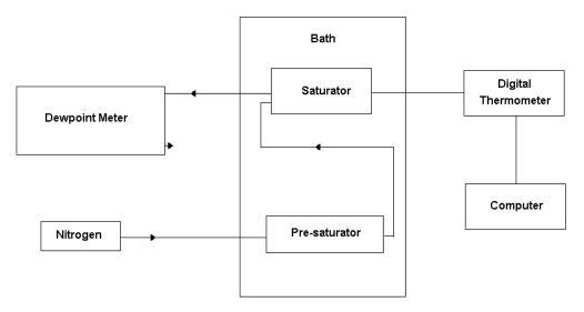
Figure3 – Schematic design of the humidity generation system
