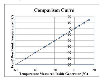
Figure 4 – Comparison check of the humidity generator with the standard dewpoint meter S4000
