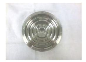
Figure 2 – View of the internal part of the humidity generator
