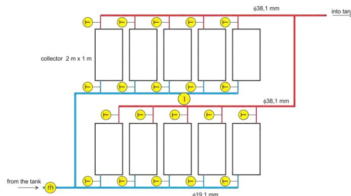
Fig. 4. Details of experimental device, parallel configuration.
