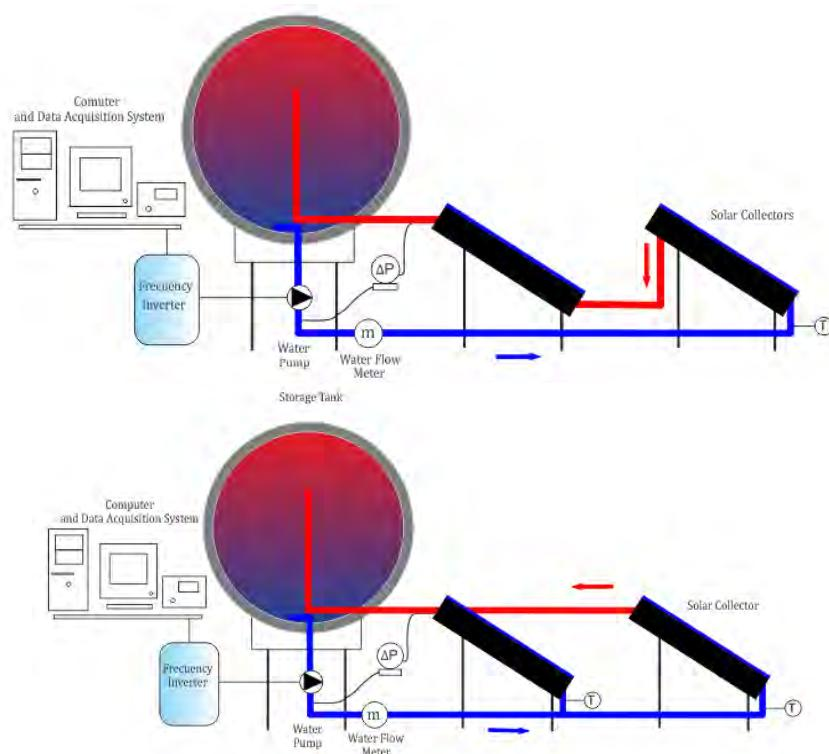
Fig.1. Solar water heating system distributions
