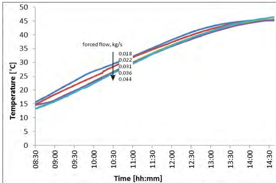
Fig. 7. Tank temperature in forced flow vs. time.
