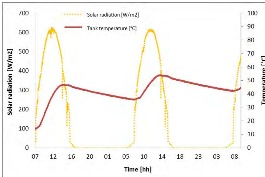
Fig. 8. Night heat loss in the tank vs. time.
