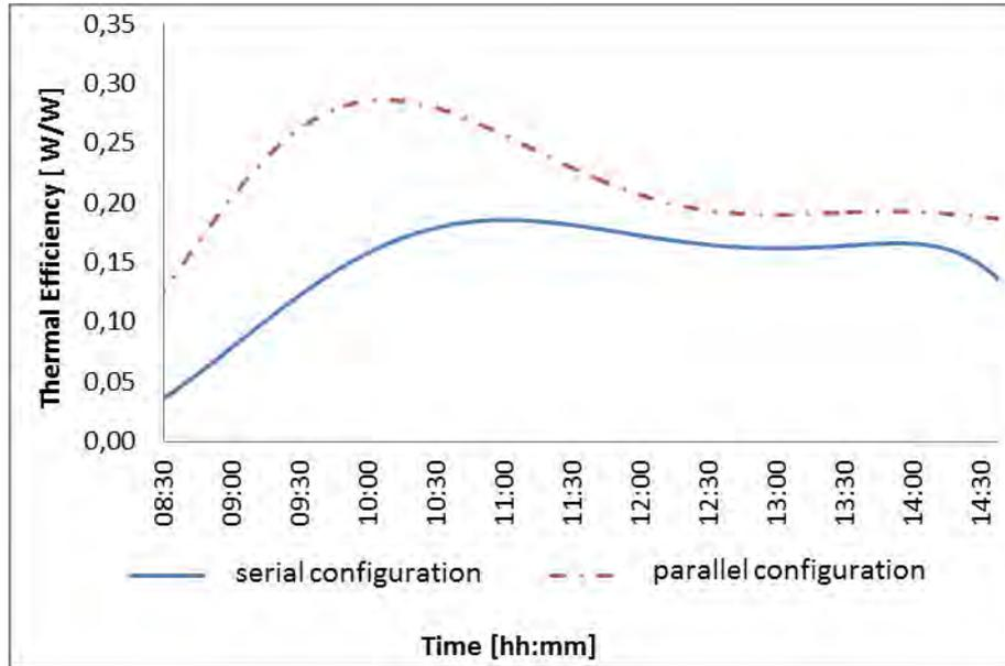
Fig. 5. Thermal efficiency in natural convection vs. time.
