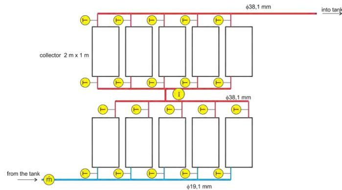
Fig. 3. Details of experimental device, serial configuration.
