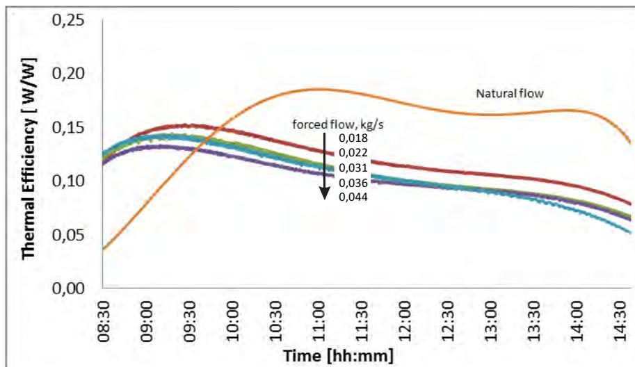
Fig. 6. Thermal efficiency in forced flow vs. time.
