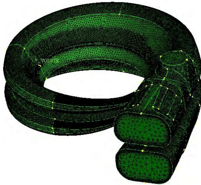
Figure 6. Volute domain mesh (2,2 millions of control volumes)
