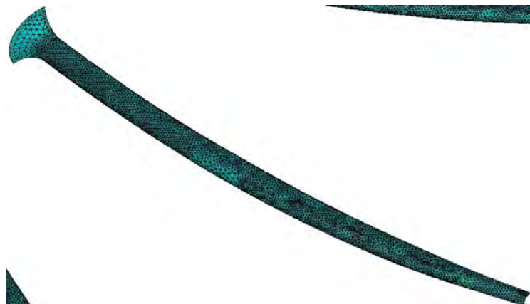
Figure 8. Refined mesh at the trailing edge of the rotor
