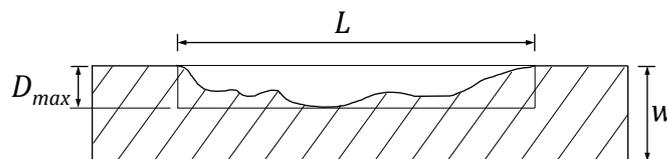
Figure 5. Corrosion defect dimensions
