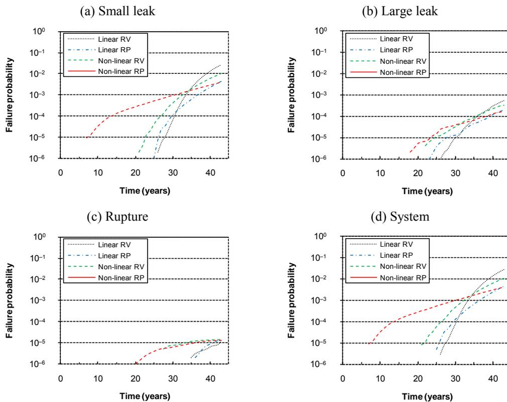
Figure 7. Time-varying failure probabilities for the example pipeline. Linear and non-linear, random variable and random process models. RV: random variable; RP: random process.
