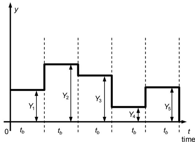
Figure 6. Realization of a Borges internal pressure load process (adapted from Melchers, 1999)
