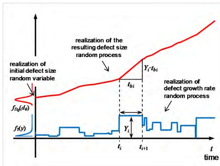
Figure 2. Construction of defect size “linear” random process, from random (variable) initial defect and Poisson square wave process defect growth rate
