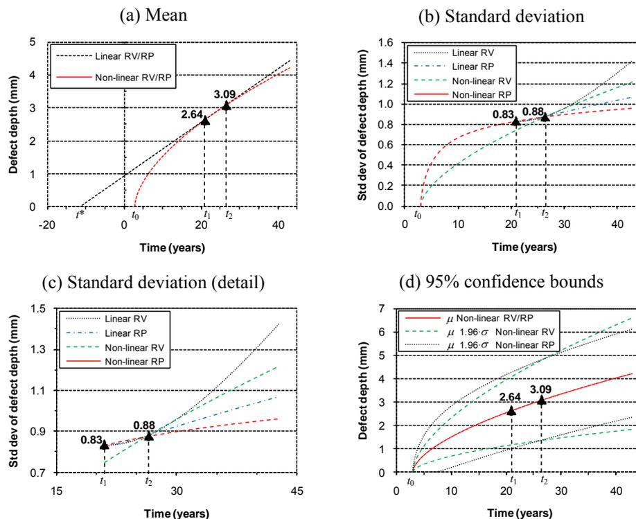
Figure 4. Time evolution of corrosion depths for different corrosion growth models, calibrated to actual data. RV: random variable; RP: random process
