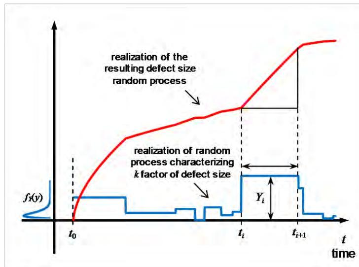
Figure 3. Construction of defect size “non-linear” random process, from Poisson square wave process characterizing proportionality factor of defect size
