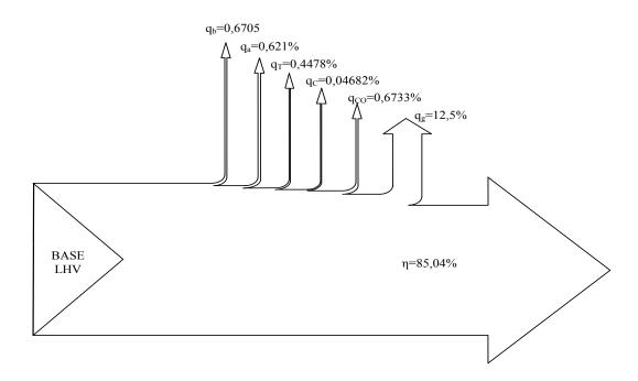
Figure 2. Sankey's diagram for the bagasse boiler efficiency (LHV as calculation base).
