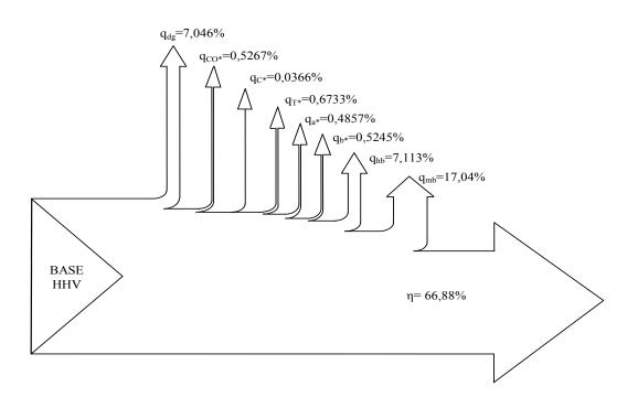
Figure 3. Sankey's diagram for the bagasse boiler efficiency (HHV as calculation base).
