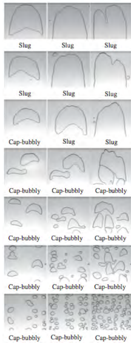
Figure 1: Two-phase upward flow structures in a narrow rectangular channel. Adapted from Shen et al. (2012).
