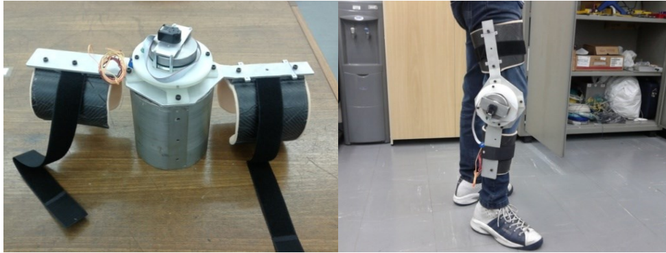
Figure 3. Knee actuation module. On the left it can be seen the final prototype and on the right is worn by a user.
