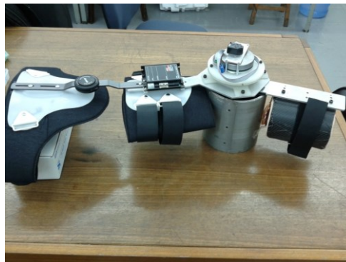
Figure 4. Exoskeleton comprising the hip orthosis linked to the knee actuation module.
