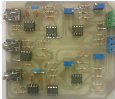
Figure2. Board of analog hardware for electromyographic signal conditioning
