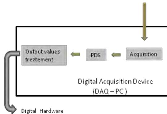
Figure 3. Scheme of analog-to-digital converter
