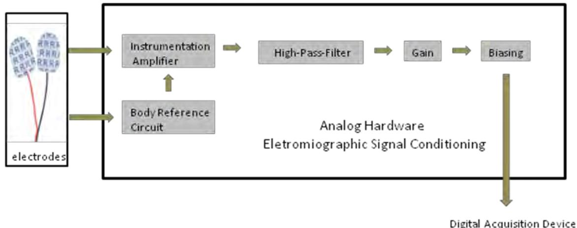
Figure 1. Scheme of analog hardware for electromyographic signal conditioning
