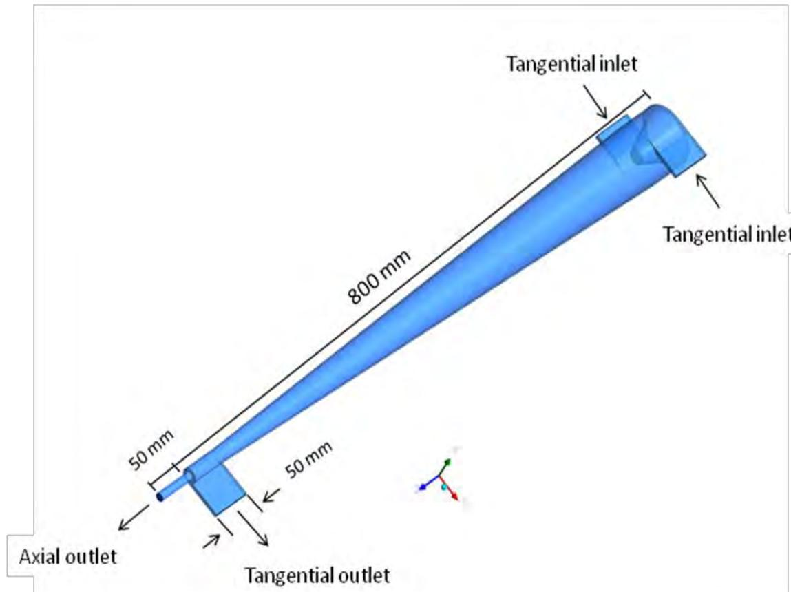
Figure 1: Representation of Cyclonic Separator
