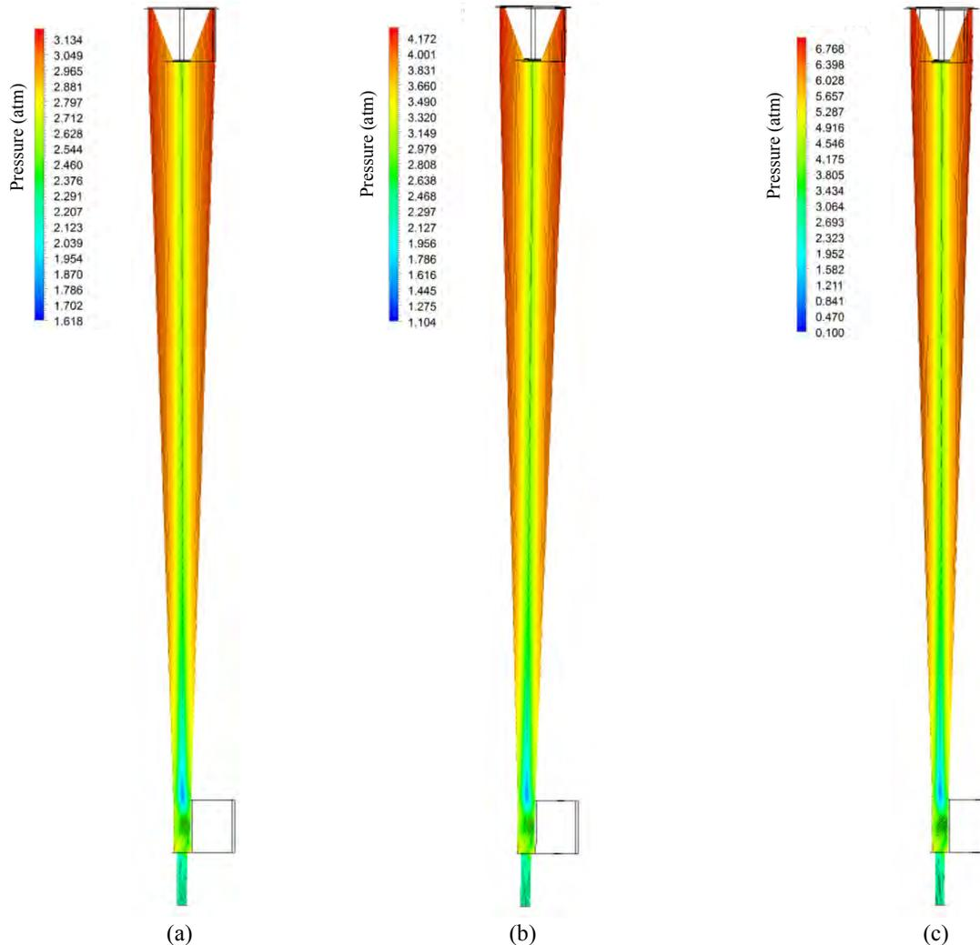
Figure 4: Representation of the pressure field on the xz planes (a) 4,5 m<sup>3</sup>/h; (b) 6,3 m<sup>3</sup>/h e (c) 9,0 m<sup>3</sup>/h
