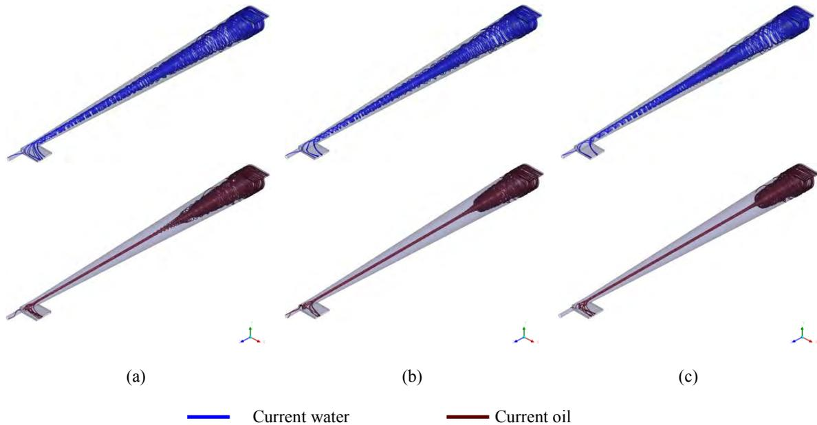
Figure 2: Flow line inside the cyclonic separator for different inlet flow (a) 4.5 m<sup>3</sup>/h; (b) 6.3 m<sup>3</sup>/h and (c) 9.0 m<sup>3</sup>/h
