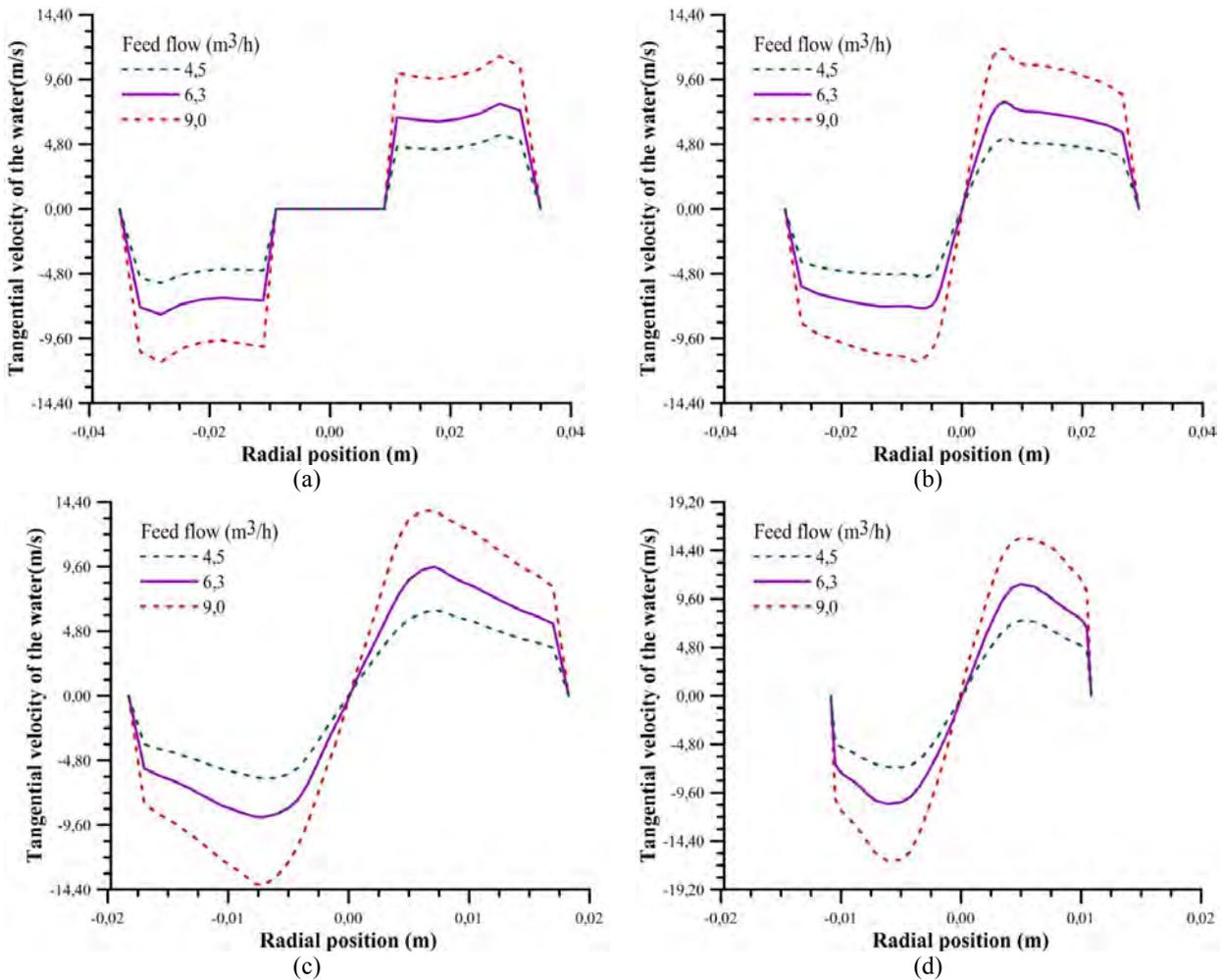
Figure 5: Analysis of the influence of rate of input into the tangential velocity profile (a) 50 mm; (b) 200 mm; (c) 500 mm e (d) 700 mm
