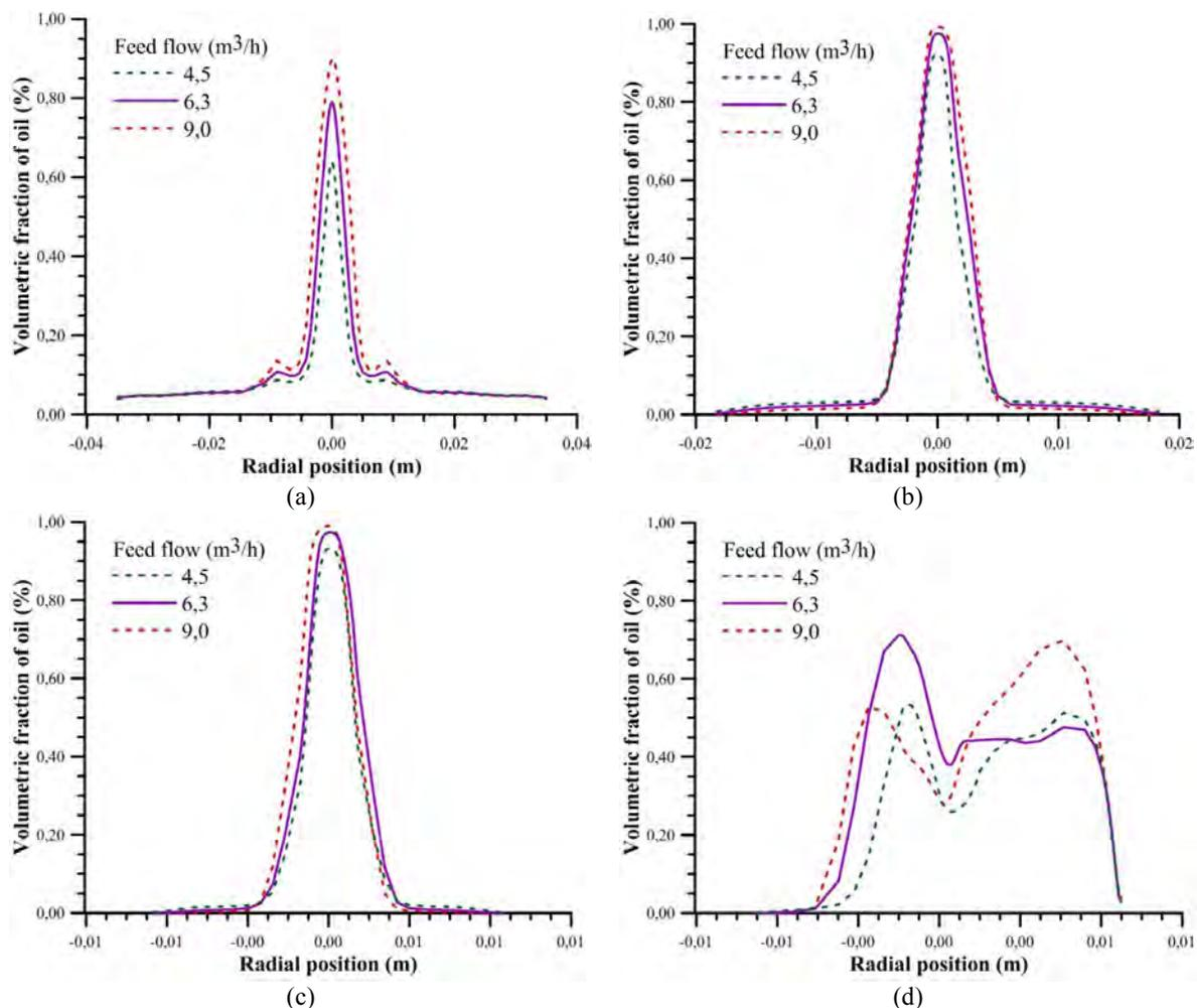
Figure 6: Analysis of the influence of input flow in equipment efficiency (a) 50mm; (b) 500 mm; (c) 700mm e (d) 775mm
