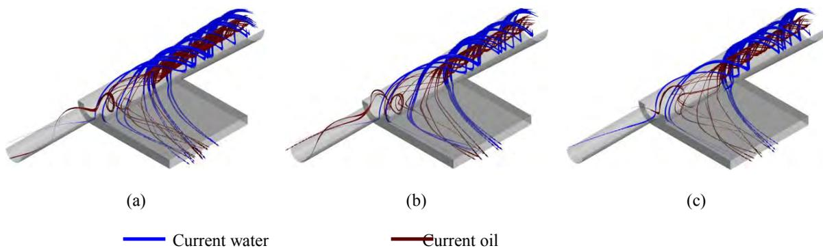
Figure 3: Flow line in the cyclonic separator outputs for different input flows(a) 4.5 m<sup>3</sup>/h; (b) 6.3 m<sup>3</sup>/h and (c) 9.0 m<sup>3</sup>/h
