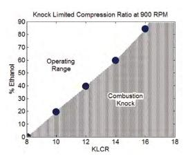
Figure 10.Experiment of a variable compression ratio engine and a variable blend of gasoline and ethanol. Source: Cooney et al (2009).
