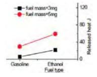
Figure 9.Comparison of fuels burn (NVO period) in stoichiometric mixtures. Source: Yang et al (2010).
