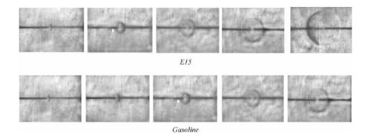
Figure 8.Flame core growth captured by schlieren camera for stoichiometric mixtures of E15 and Gasoline. Source: Liao et al (2005).
