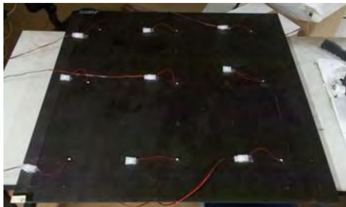
Figure 1. Composite carbon/epoxy plate instrumented with piezoelectric sensors.
