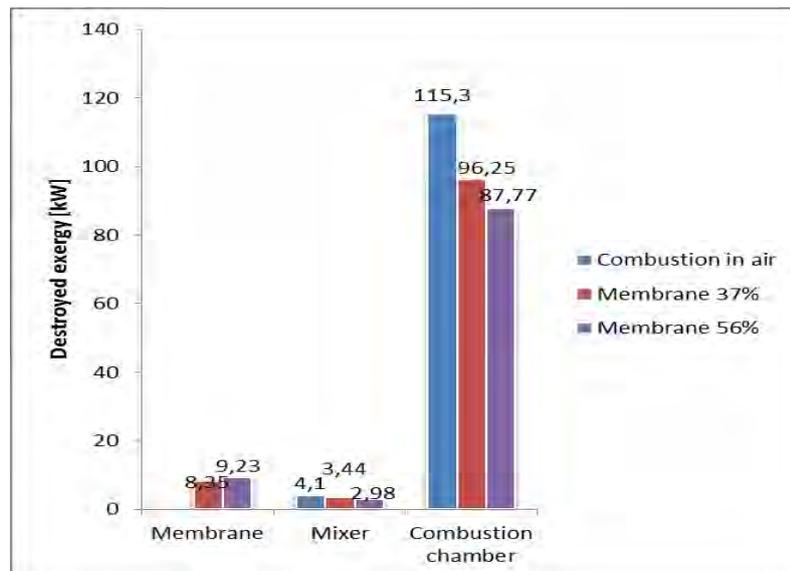
Figure 9. Destroyed exergy of the various components for different modes of operation.
