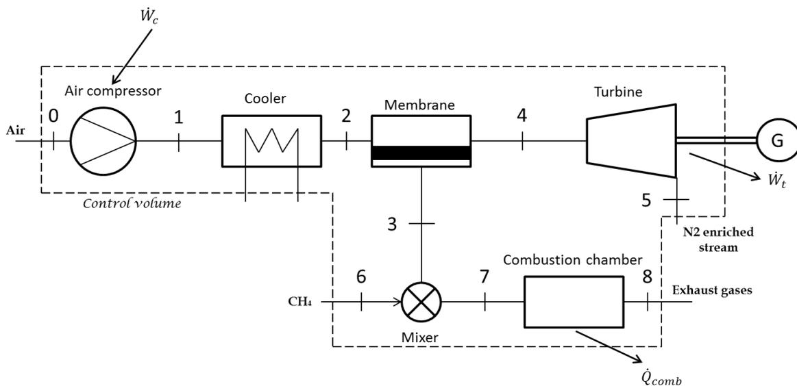
Figure 1. Schematics for OEC system with oxygen enrichment unit
