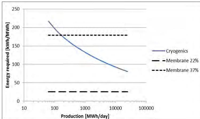
Figure 12. Energy consumption for the production of 1MWh of heat as a function of the production per day, for various techniques of oxidant production: cryogenics and membrane of selectivity 8. Data for cryogenics came from (Kauranen 2008).
