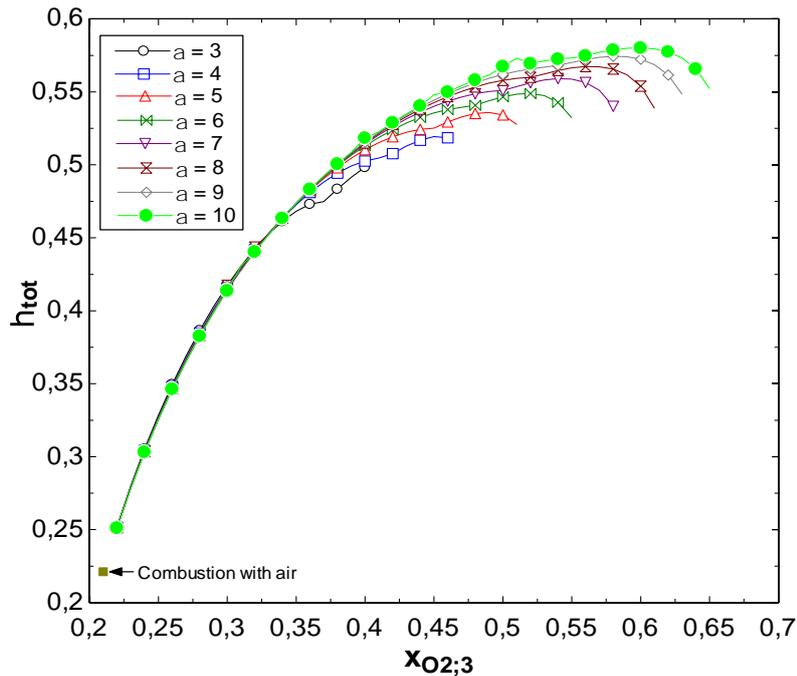
Figure 5. System efficiency for various selectivities as a function of enrichment.
