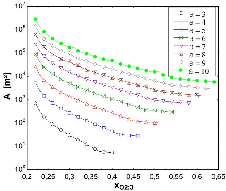
Figure 4. Optimum membrane area as a function of enrichment level.
