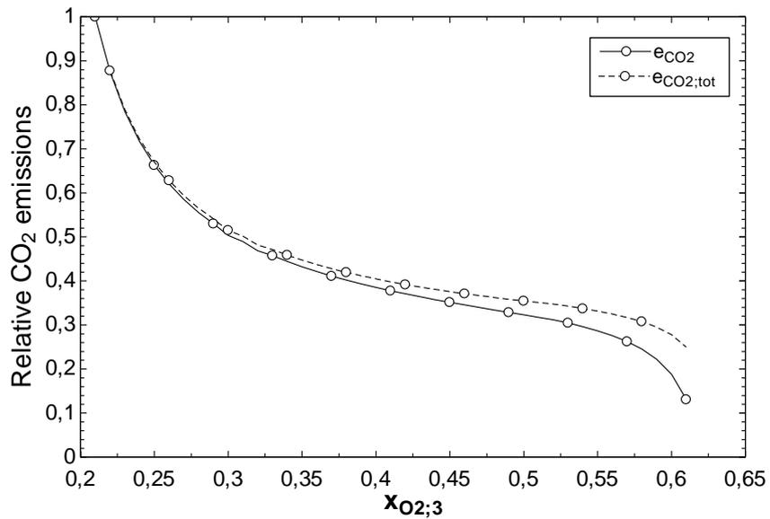
Figure 6. Relative specific CO<sub>2</sub> emissions  $e_{CO_2}$  and total relative specific CO<sub>2</sub> emissions  $e_{CO_2,tot}$ , for a membrane of selectivity 8 as a function of oxygen enrichment.
