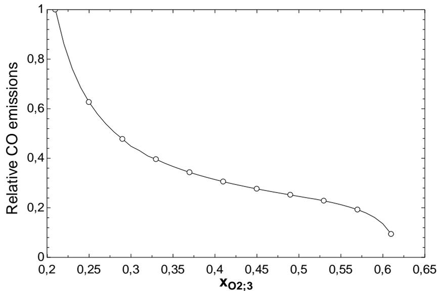
Figure 7. Relative specific CO emissions for a membrane of selectivity 8 as a function of enrichment
