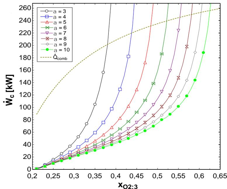
Figure 3. Compressor power as a function of enrichment level for membranes with various selectivities and variable surface area (according to Fig. 4).
