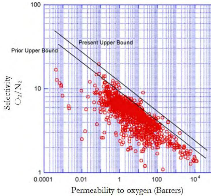
Figure 2. Upper bound correlation for  $\text{O}_2/\text{N}_2$  separation (Robeson 2008).
