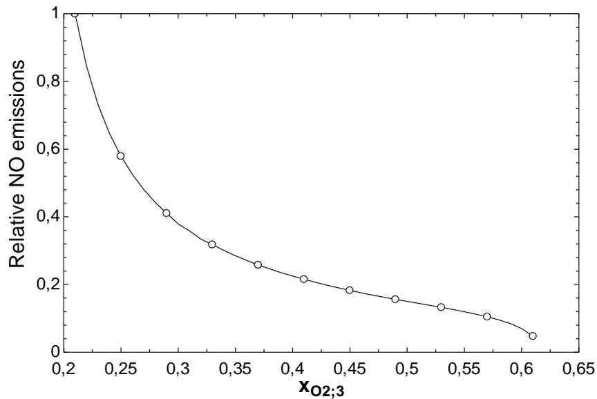
Figure 8. Relative specific NO emissions for a membrane of selectivity 8 as a function of enrichment.
