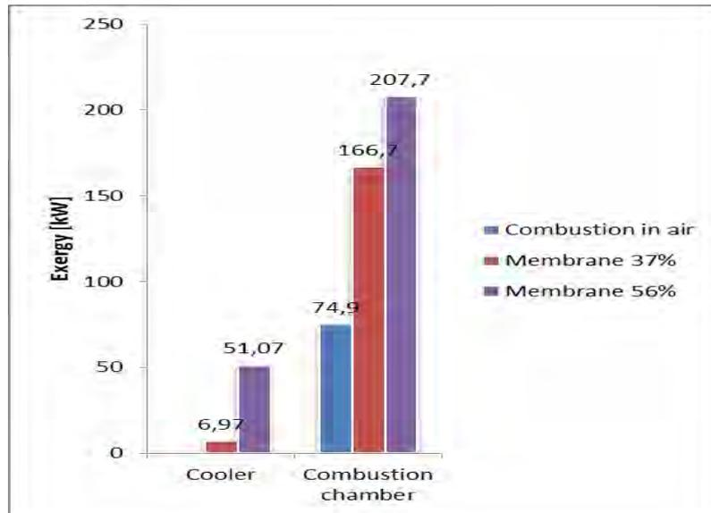
Figure 10. Exergy transfer by heat in the various components for different modes of operation
