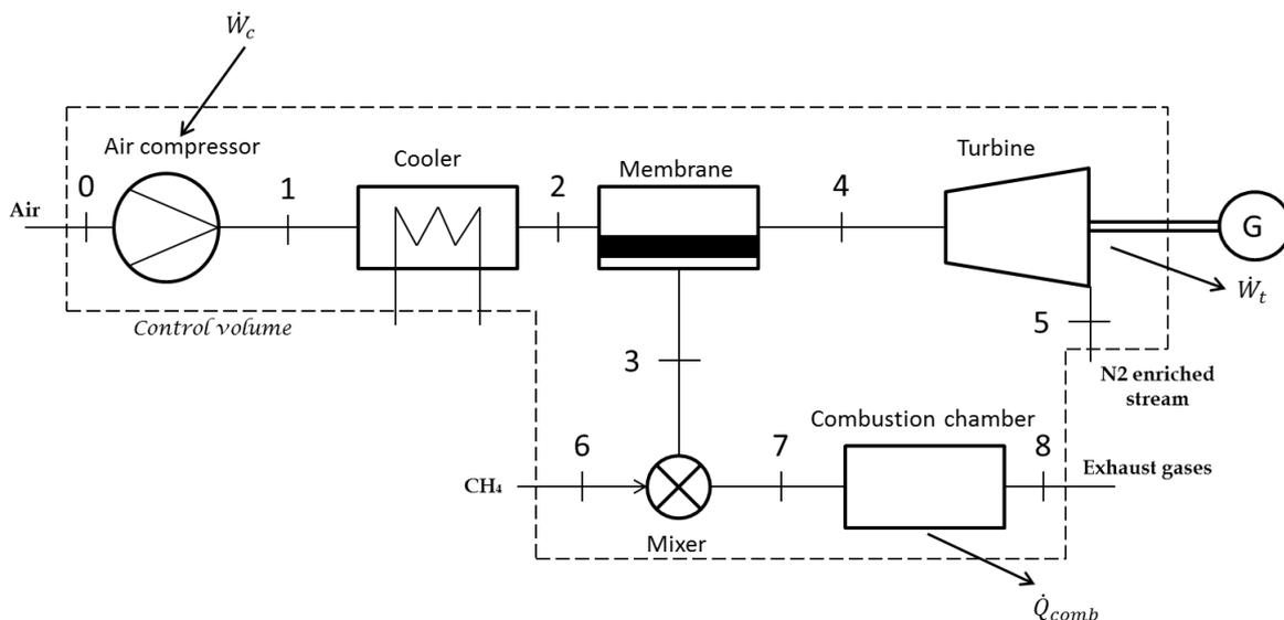
Figure 1. Schematics for OEC system with oxygen enrichment unit
