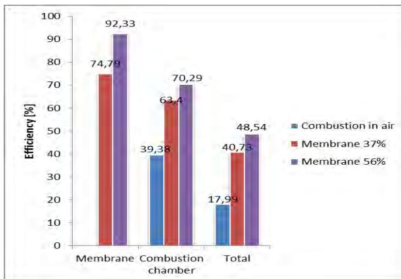
Figure 11. Exergetic efficiency of main components for different modes of operation.
