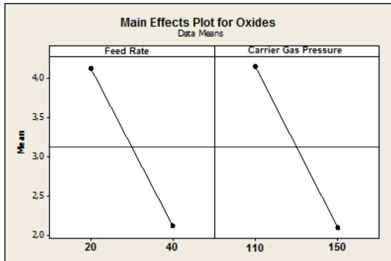
Figure 5. Main effects plots of feed rate and carrier gas pressure for oxide contents.
