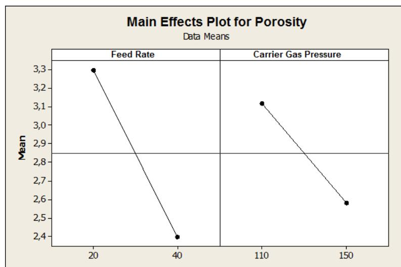
Figure 4. Main effects plots of feed rate and carrier gas pressure for porosity.
