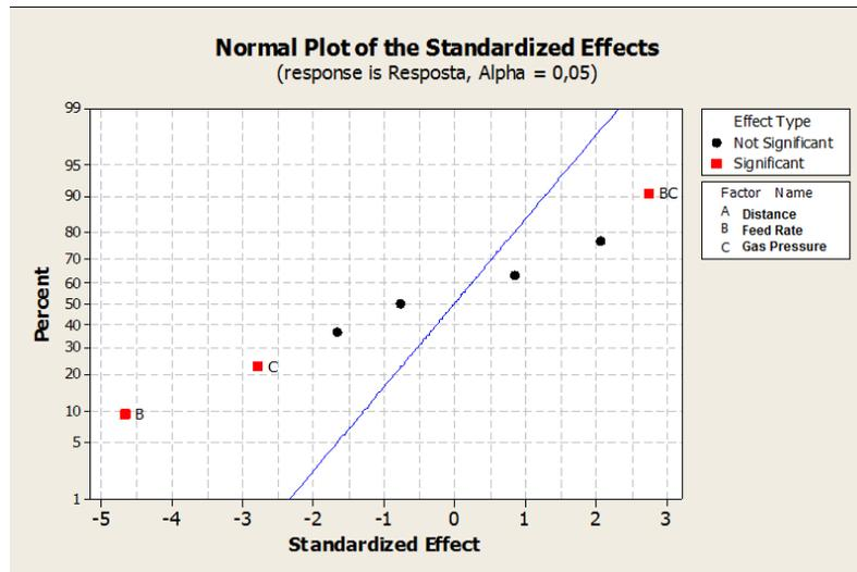
Figure 3. Normal plot of the standardized effects for the oxide contents.
