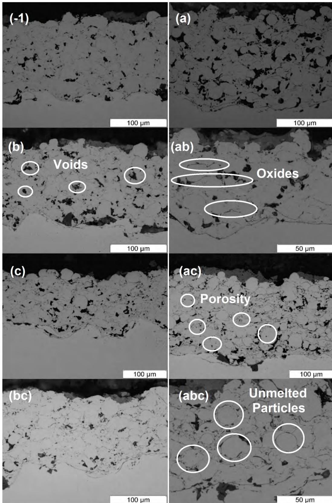
Figure 1. Cross section of the coatings for each treatment analyzed- Replica 1. Featured in the images are the pores, voids, oxides and unmelted particles which occurred during deposition by HVOF.
