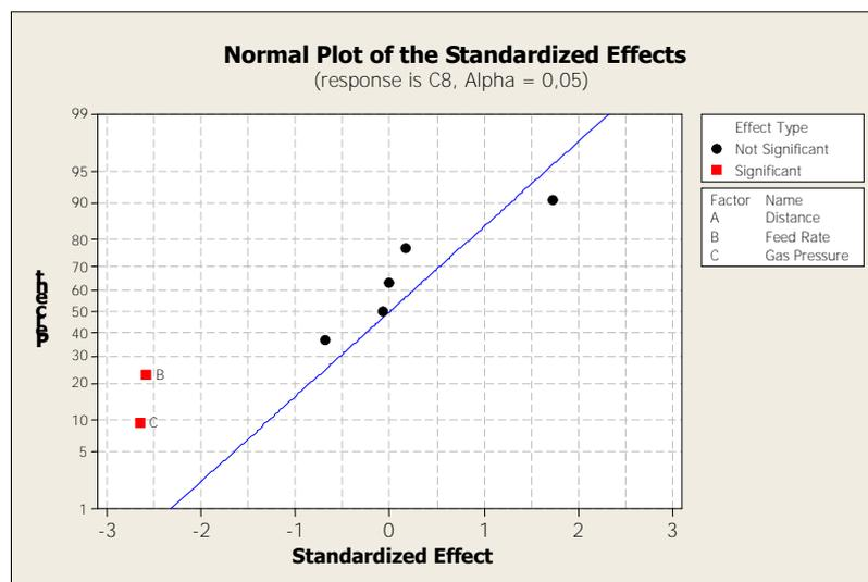
Figure 2. Normal plot of the standardized effects for the porosity.
