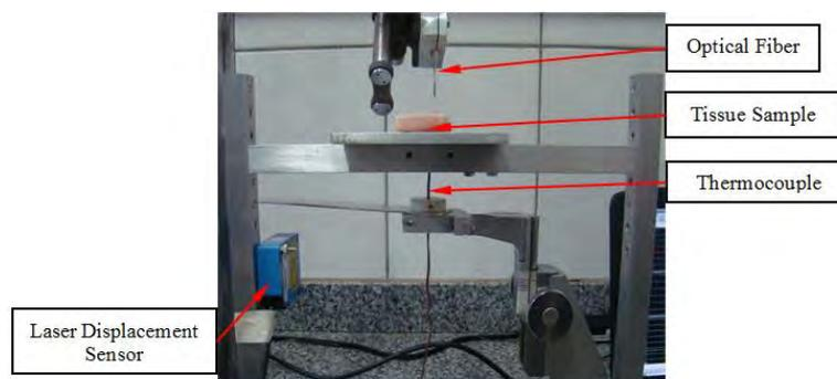
Figure 6 – Thermocouple used to measure temperature of sample skin subject a laser radiation.
