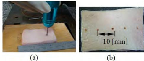
Figure 5- Sample preparation for evaluation of temperature (a) drilling of skin to pass the thermocouple (b) sample ready to be tested.
