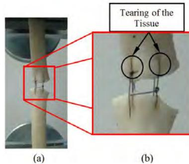
Figure 10- Tensile test on sutured sample. (a) sample placed between the grips (b) enlargement at region highlighting the tearing of the tissue.
