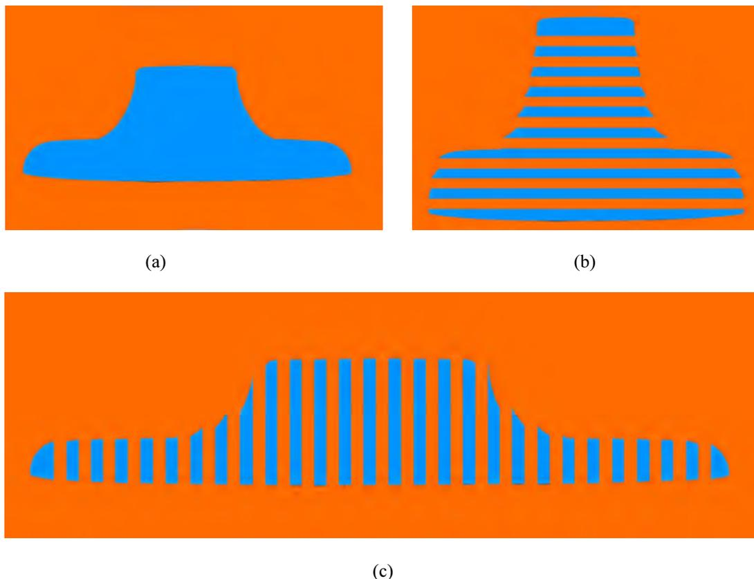
Figure 3: (a) Model, (b) model with overlapping layers on vertical direction and (c) with overlapping layers on horizontal direction.
