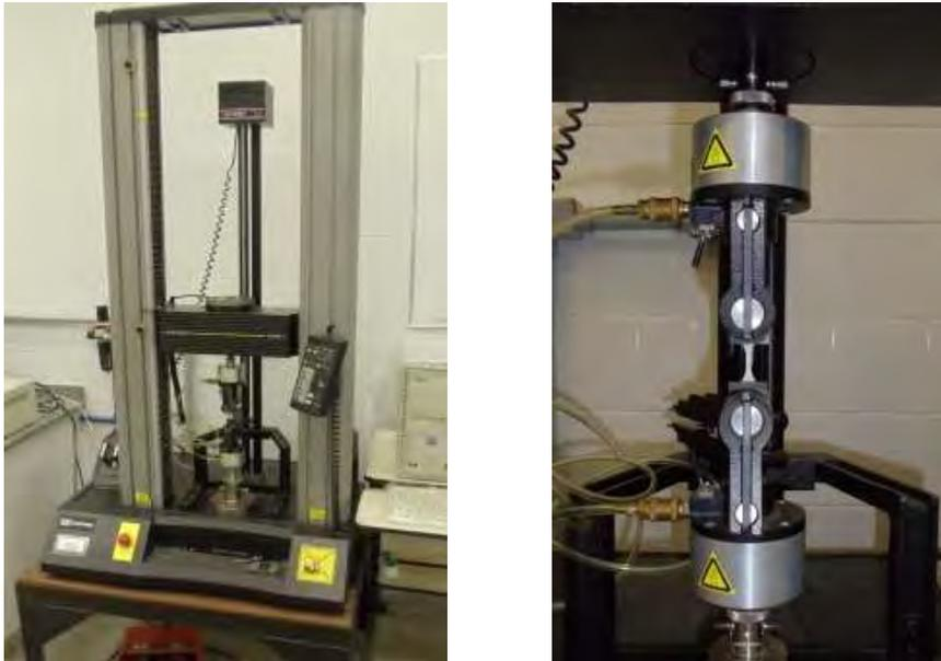
Figure 5. (a) Tensile test set-up and (b) detail of the specimen fixed by the pneumatic claws.
