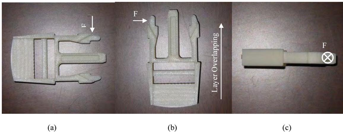
Figure 11. Three different positions of the beams connector for the same overlapping layer orientation.
