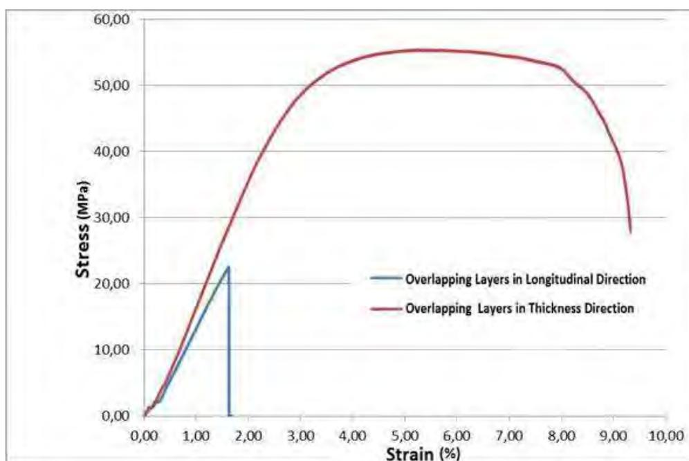
Figure 9. Graphs Flexure Stress x Strain plotted with data from bending tests with both types of specimens.
