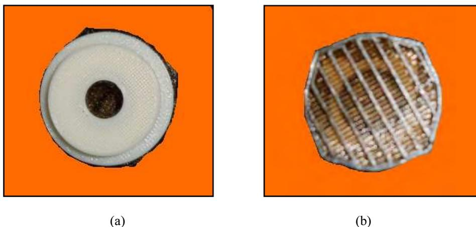
Figure 2. (a) The support material in the hole (void) of the model and (b) on the back of the model.
