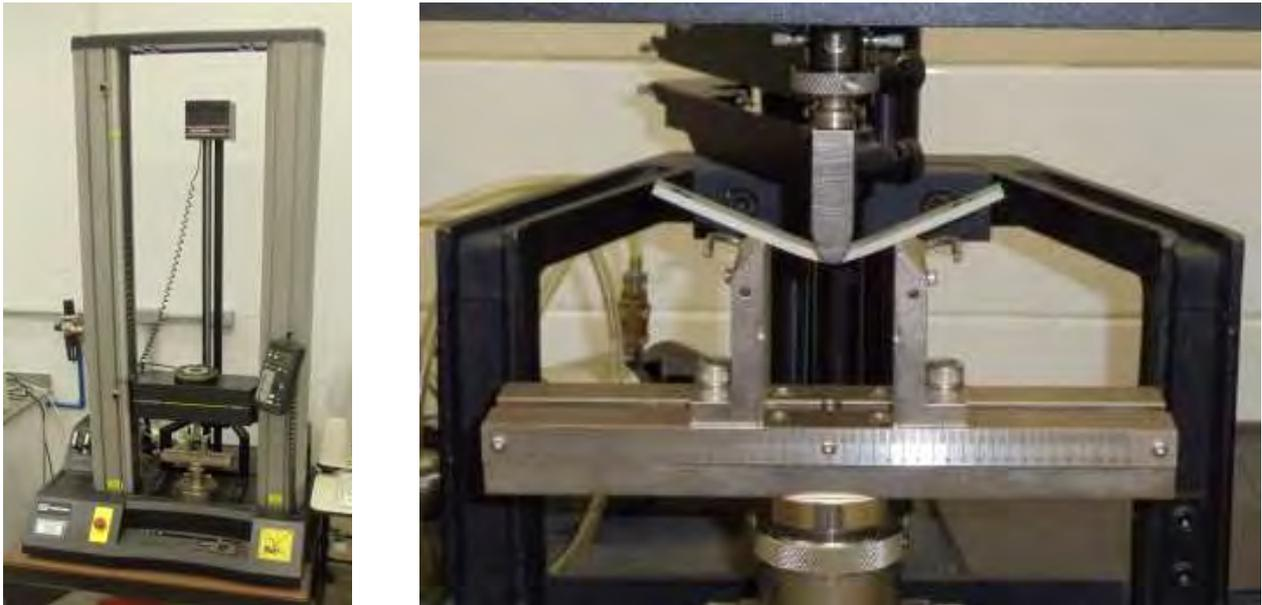
Figure 8. Experimental set-up for bending tests.
