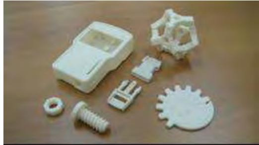
Figure1. Products printed by FDM at PRO-SME laboratory.
