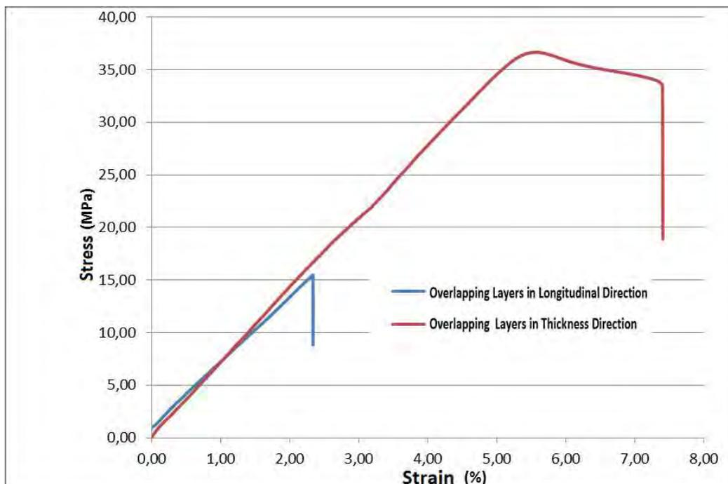
Figure 6. Graphs Stress x Strain plotted with data from tensile tests with the two types of specimens.
