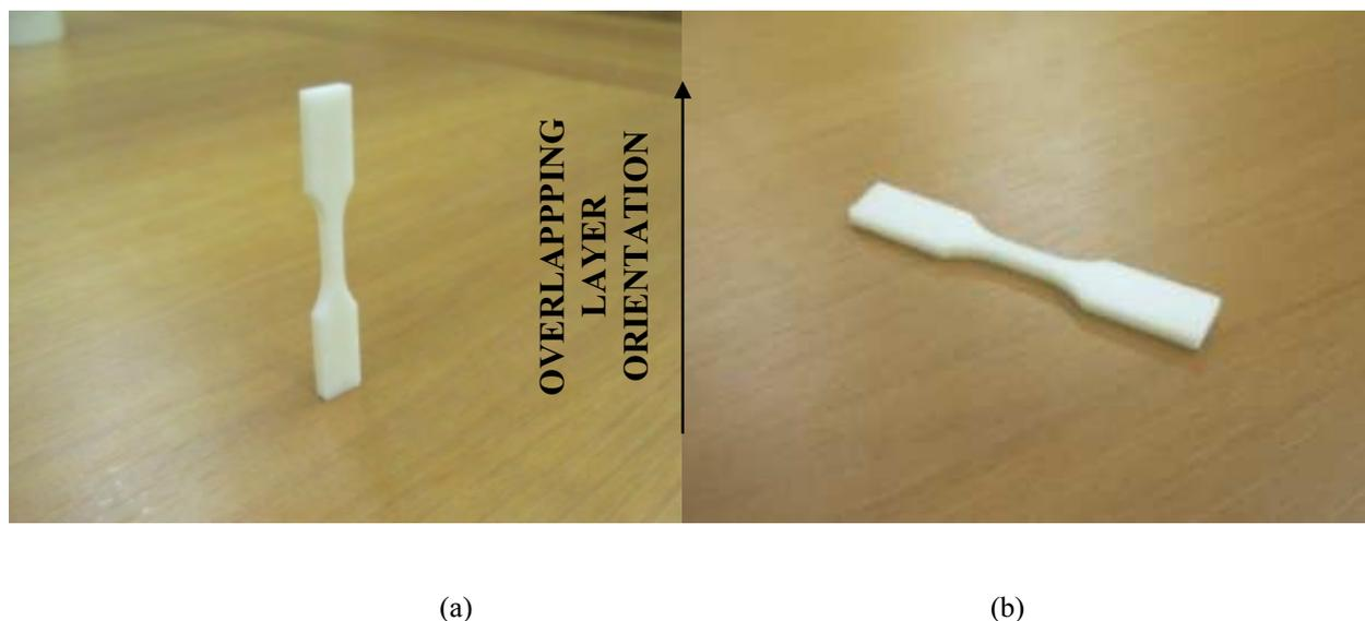
Figure 4 – (a) Specimens printed with overlapping layers in the longitudinal direction and (b) in the thickness direction.
