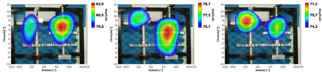
Figure 4. Sound maps at different instants of time to machine running in fault condition at 6300 Hz.
