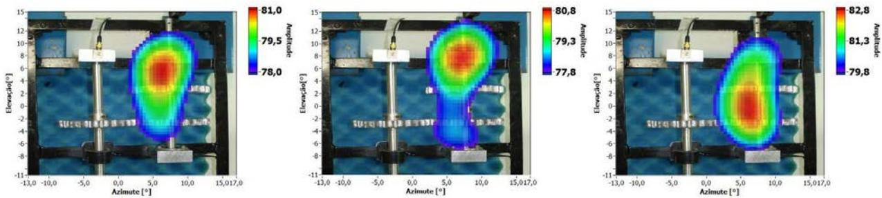
Figure 3. Sound maps at different instants of time to machine running in normal conditions at 6300 Hz.
