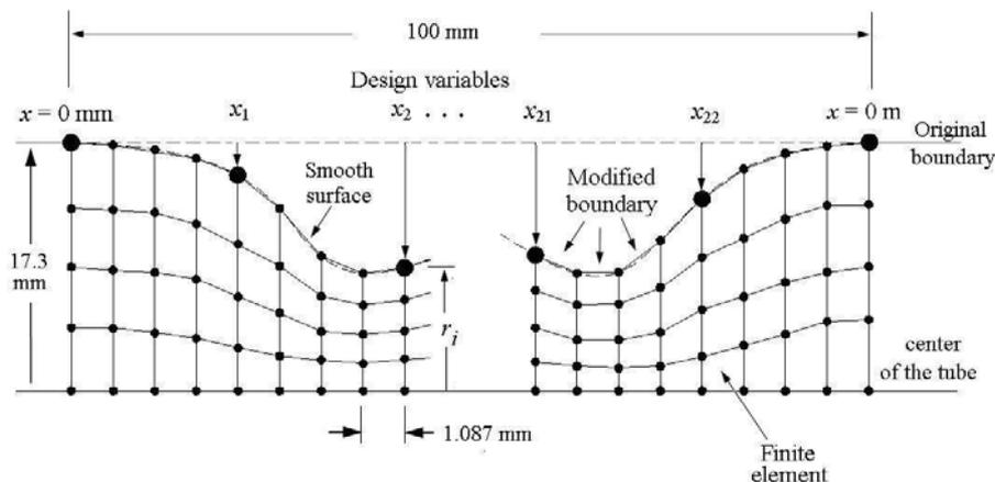
Figure 1. Definition of the optimized tube profile and the design variables
