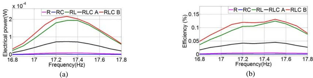
Figure 8. Comparison between R, RC, RL and RLC circuits results: a) Generated electrical power; b) Efficiency.
