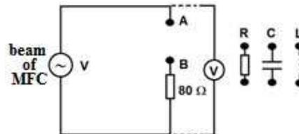
Figure 4. Electrical circuit used in the tests. R – resistor, C – capacitor, L – inductor.
