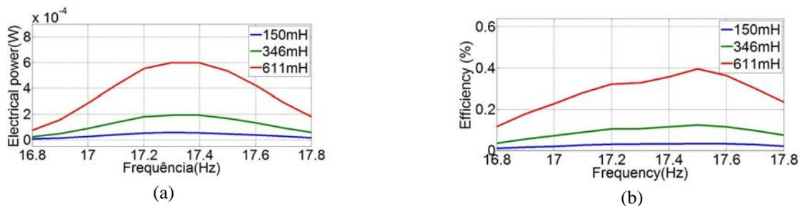
Figure 8. RL circuit influence results: a) Generated electrical power; b) Efficiency.
