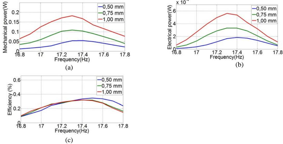
Figure 5. Results for different base oscillation amplitudes: a) Supplied mechanical power; b) Generated electrical power; c) Efficiency.
