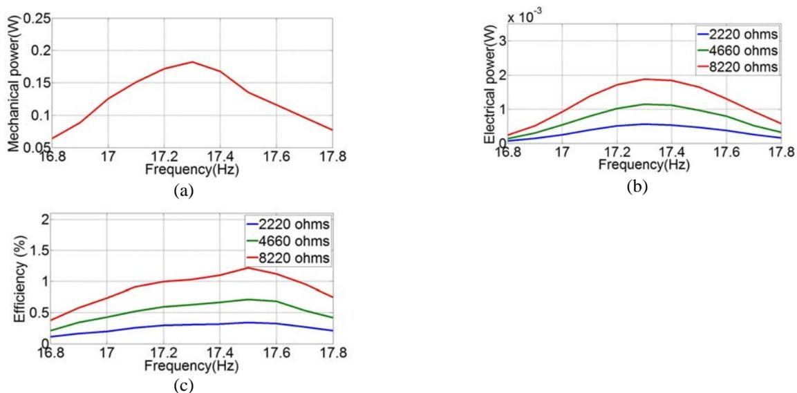
Figure 6. R circuit influence results: a) Supplied mechanical power; b) Generated electrical power; c) Efficiency.
