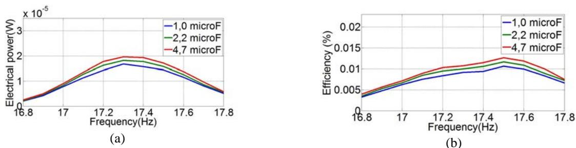
Figure 7. RC circuit influence results: a) Generated electrical power; b) Efficiency.
