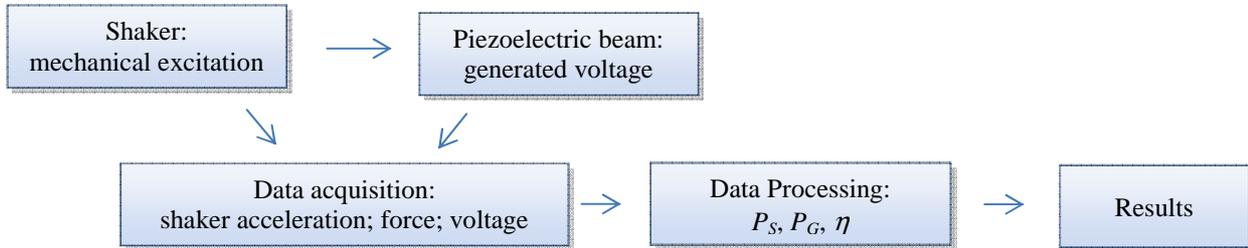
Figure 3. Flow diagram of experimental procedure.
