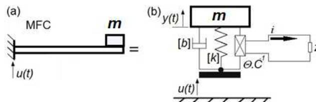
Figure 1. Piezoelectric power harvesting device. (a) MFC piezoelectric beam, (b) Equivalent mass-spring-damper system coupled to a circuit (similar to Priya & Inman, 2008; Triplett & Quinn, 2009).
