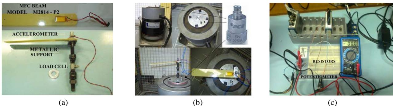
Figure 2. Experimental setup details. a) Piezoelectric beam attached to metallic support, accelerometer and force sensor; b) Beam attached to the shaker and control accelerometer; c) Protoboard.
