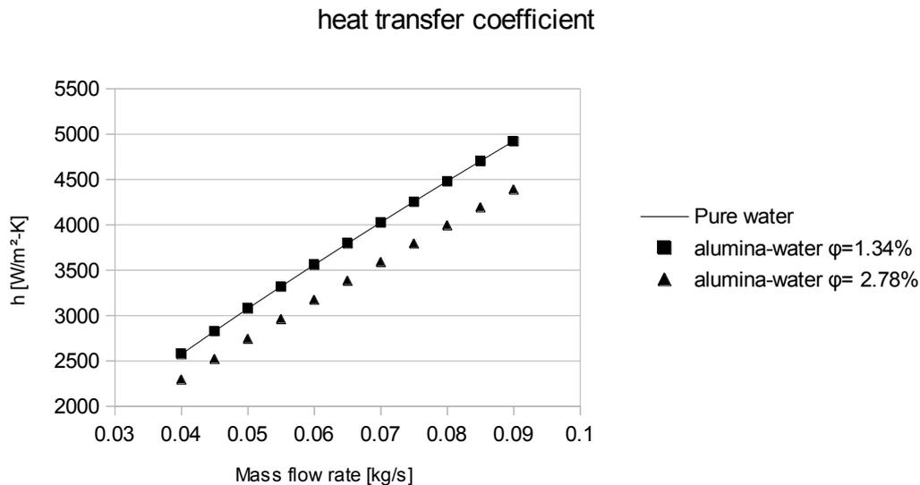
Figure 4. Comparison between heat transfer coefficient alumina-water nanofluids and water at the same mass flow rate
