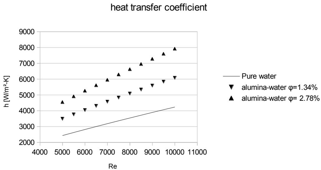
Figure 3. Comparison between heat transfer coefficient alumina-water nanofluids and water at the same Reynolds number
