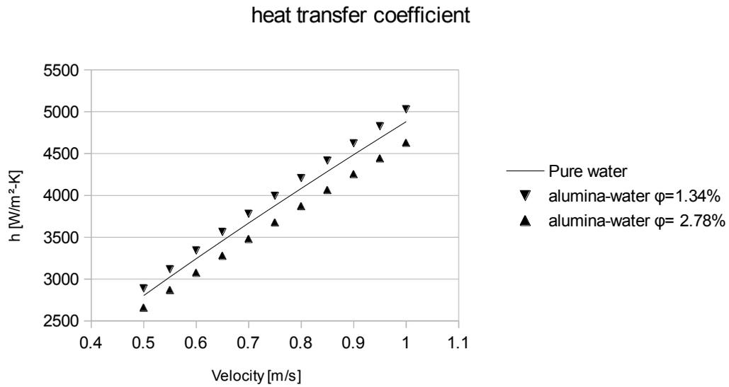
Figure 2. Comparison between heat transfer coefficient alumina-water nanofluids and water at the same mean velocity
