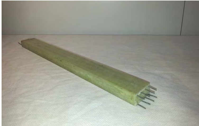
Figure 8. SMAHC beam ready to be instrumented for the bending test
