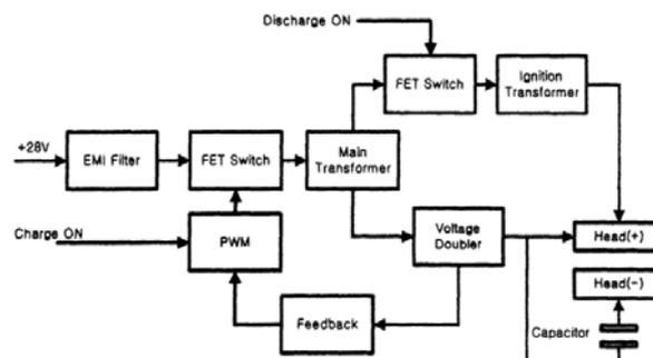
Figure 5. (Shin *et al.*, 2005) Power Processing Unit scheme.
