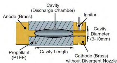
Figure 4. (Uezu *et al.*, 2005) Coaxial PPT diagram.
