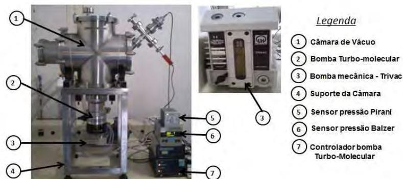
Figure 6. PPT Facility of LCP/INPE.
