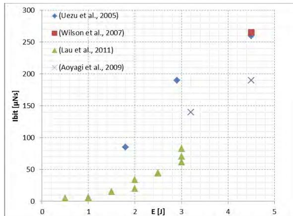
Figure 3. Demonstration of the Coaxial PPT performance at very low energy levels.
