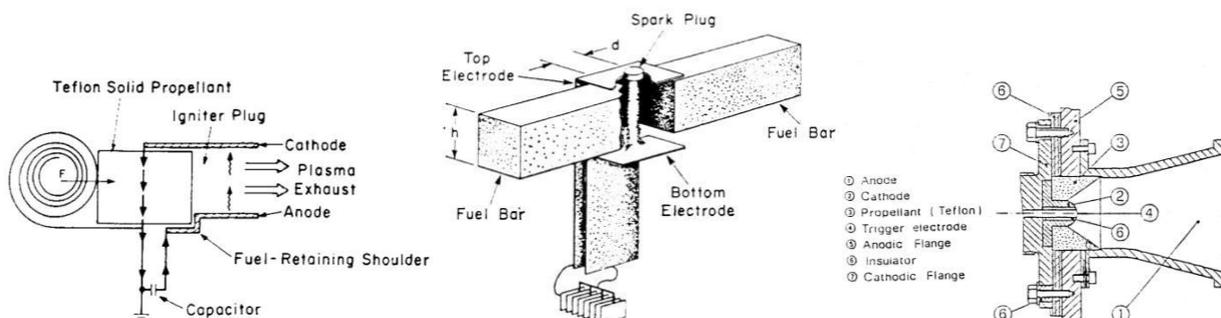
Figure 1. (Gessini *et al.*, 2005) a) (Left) Breec-fed PPT; b) (Center) Side-fed PPT; c) (Right) Coaxial PPT.
