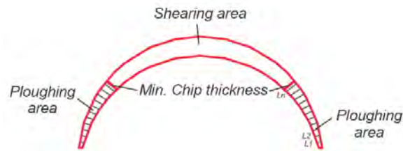
Figure 2. Shearing and ploughing areas when a_c=2R=D (Bayesteh et al. , 2013).
