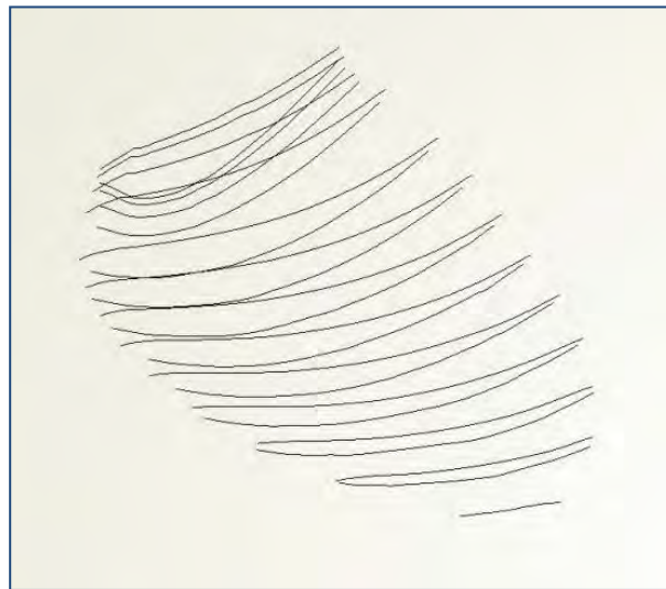
Figure 11. Curves resulting from the intersection of the cylinders and the blade's surfaces
