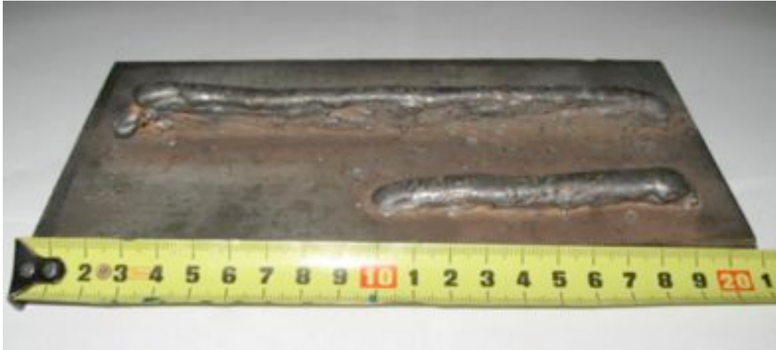
Figure 4. Sample to be studied, manufactured with rapid prototyping by arc welding method (upper sample).
