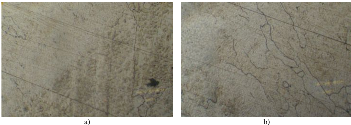
Figure 14. Microstructure of the fusion zone between adjacent beads (x300): a) boundary between fusion zone and bead; b) fusion zone.
