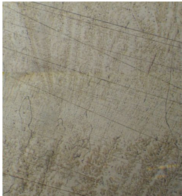
Figure 16. Fusion zone of adjacent beads in weld metal.
