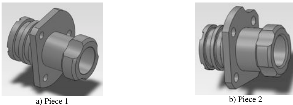
Figure 1. The body and the flange of valve block of the rocket engine gas-hydraulic drive unit.
