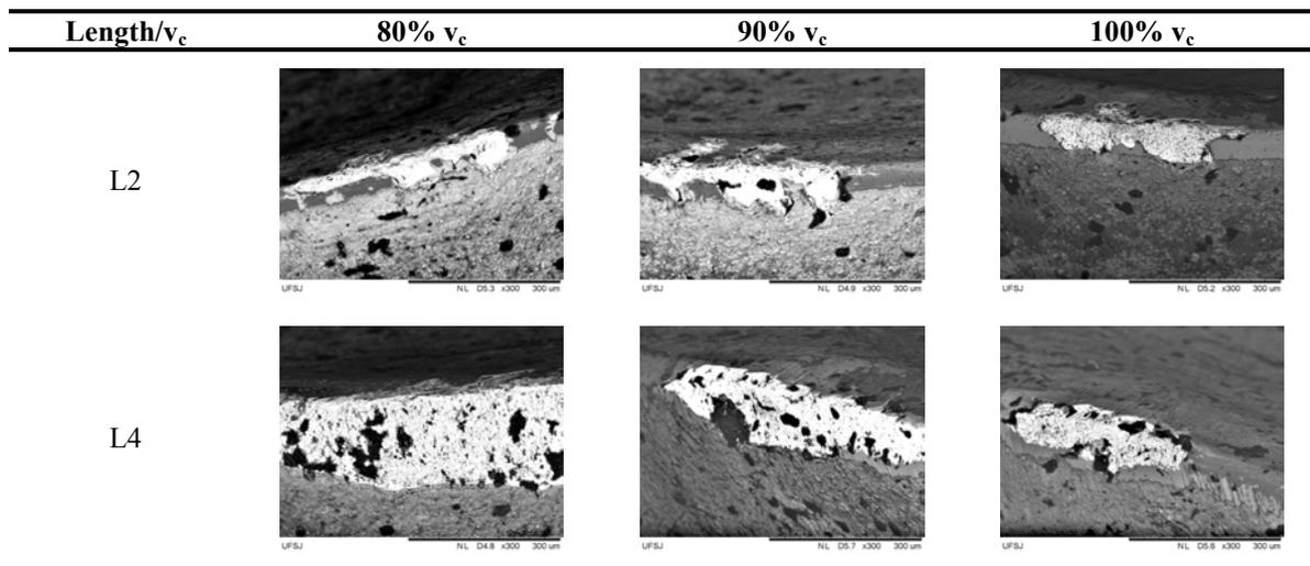
Figure 14. Secondary cutting edge of the tool T1.
