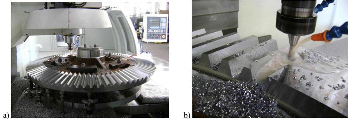
Figure 3. a) Machining Center Travis M2000; b) Installation of the tool.
