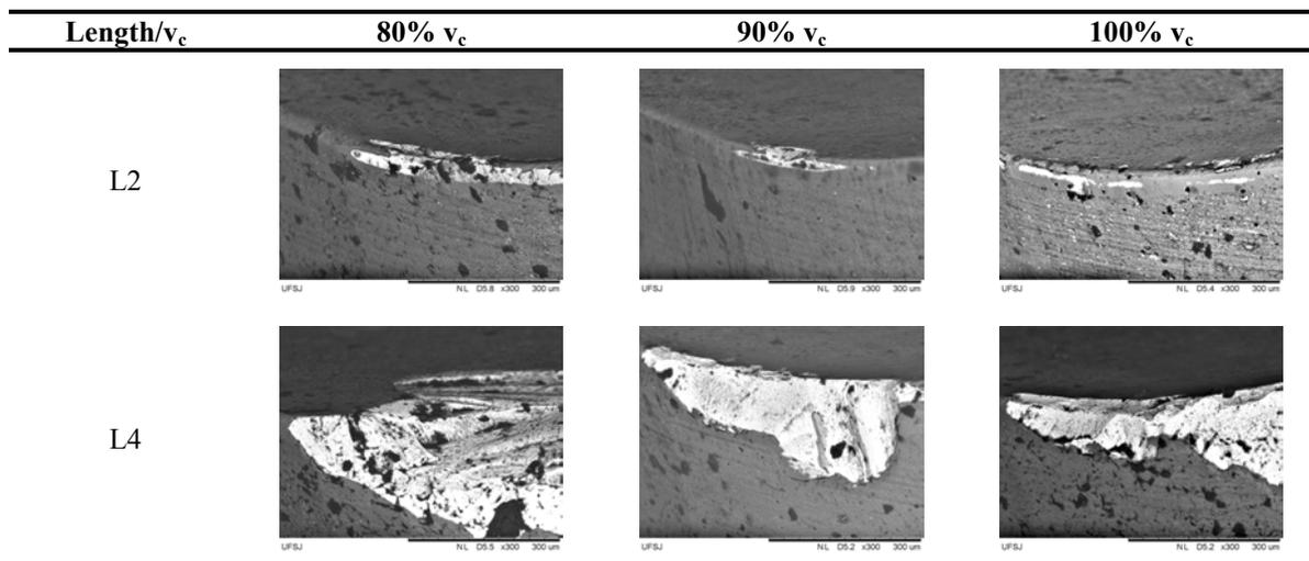
Figure 15. Secondary cutting edge of the tool T2.
