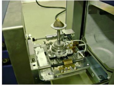
Figure 7. Fixing tool in scanning electron microscope.
