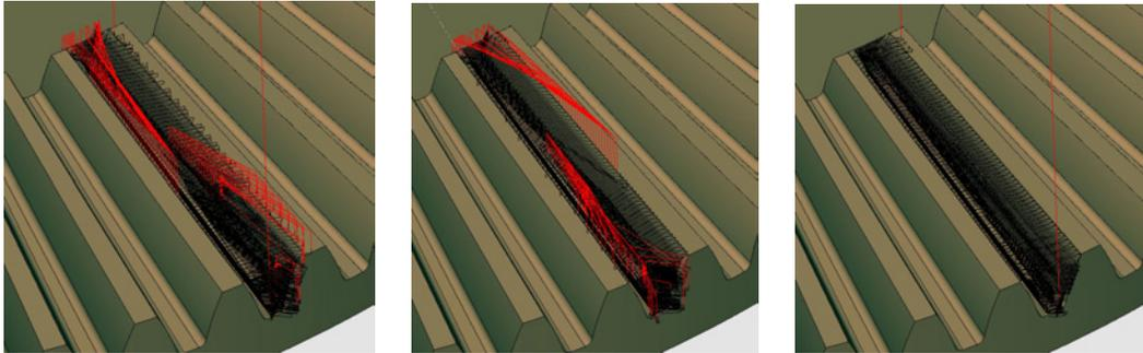
Figure 1. Different strategies in simulated machining CAM software.
