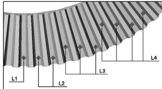
Figure 5. Determination of cut lengths.
