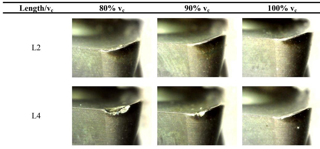
Figure 12. Secondary area off tool T2.
