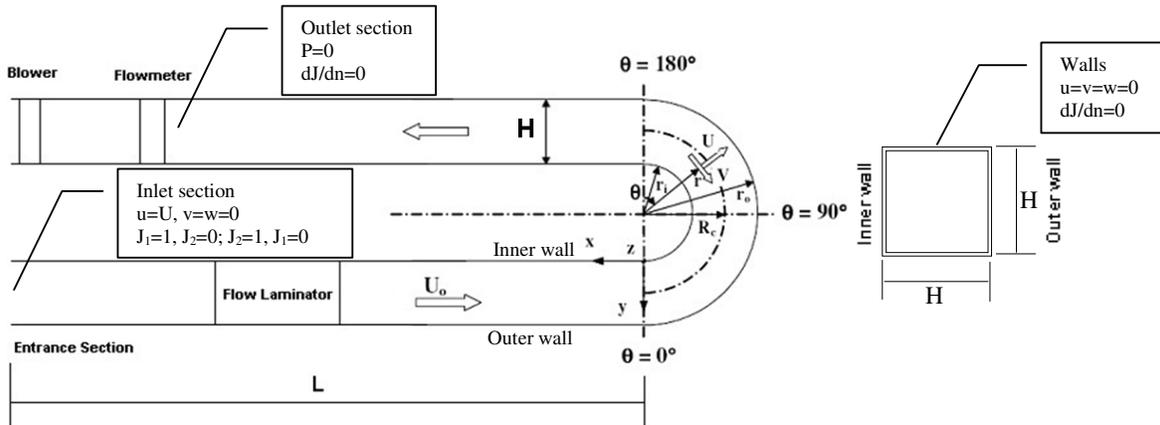
Figure 1. Problem geometry and boundary conditions for U-bend flow problem. Plan and cross section view.
