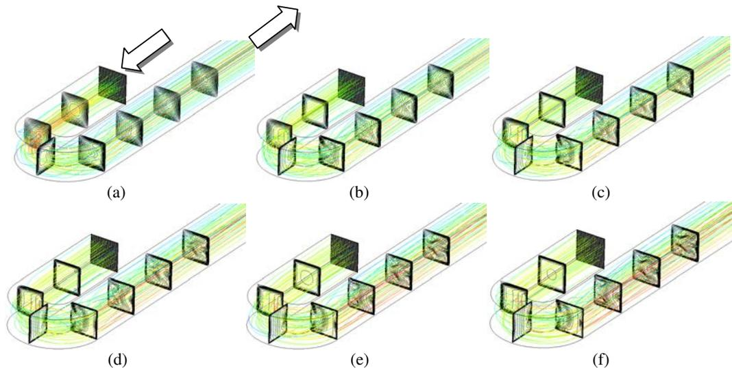
Figure 5. 3D streamlines and cross section iso-velocity. Re=100(a), 500(b), 1000(c), 1500(d), 2000(e), 2500(f)
