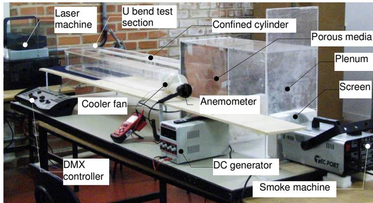
Figure 4. Workbench arrangement for flow visualization on U Duct and cylinder confined configurations
