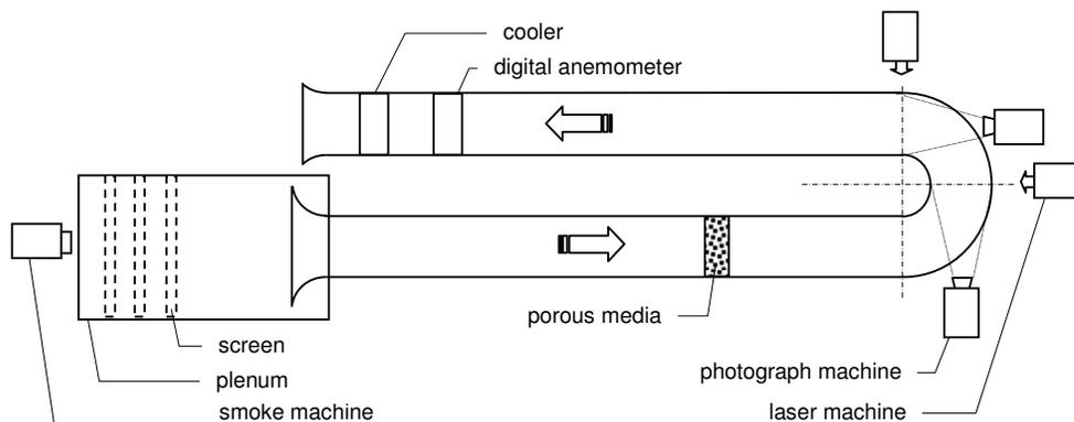
Figure 3. Experimental arrangement used to flow visualization.
