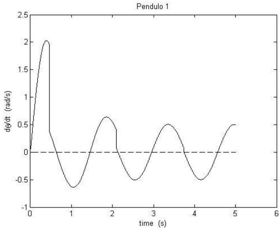
Figure 3 - The angular velocity of the pendulum.
