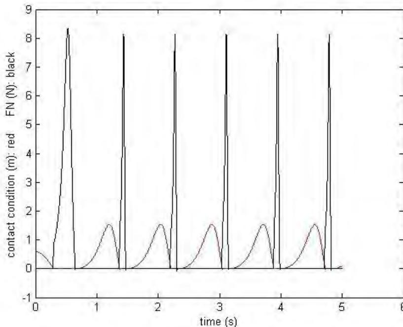
Figure 5 - The contact condition in red and the contact force in black.
