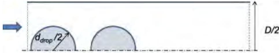
Figure 1: Sketch of the flow domain with two oil drops
