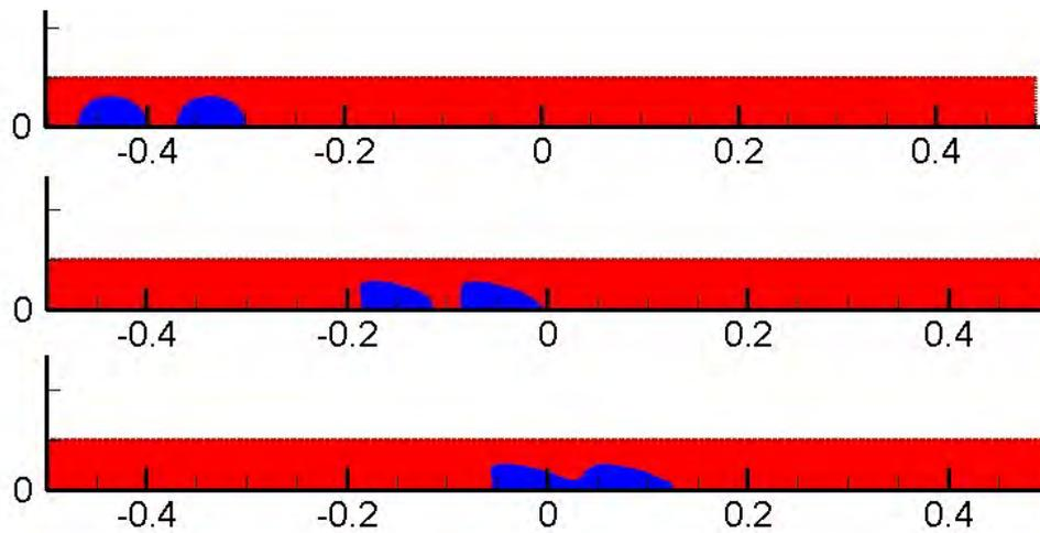
Figure 6: Evolution of the drops with  $Ca = 0.75$
