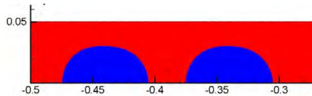
Figure 3: Initial level-set function of a pair of drops  $30\mu\text{m}$  distant of each other
