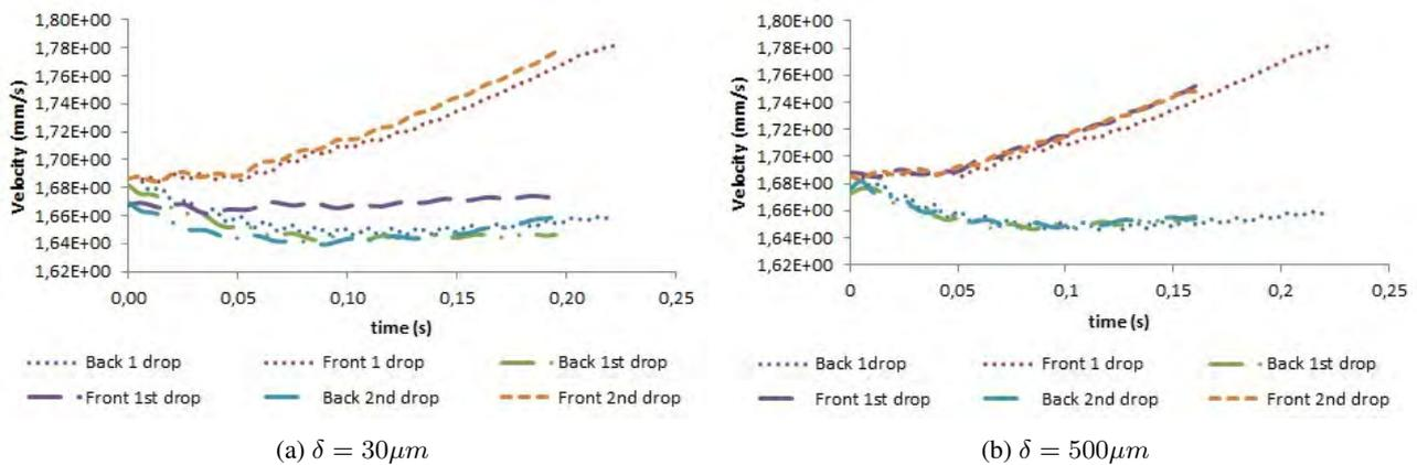
(a)  $\delta = 30\mu\text{m}$ (b)  $\delta = 500\mu\text{m}$ Figure 7: Velocity of the extremities of the drops at  $Ca = 0.75$
