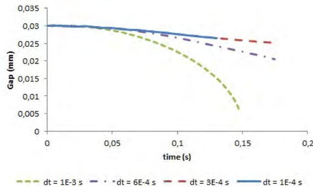
Figure 4: Gap between drops with different values of time step  $\Delta t$  with  $Ca = \infty$
