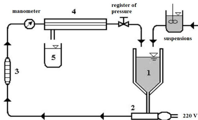
Figure 2. Schematic drawing of the experimental apparatus: (1) jacketed fluid container; (2) pump; (3) flowmeter; (4) covering module with membrane tubular; (5) permeate outflow.
