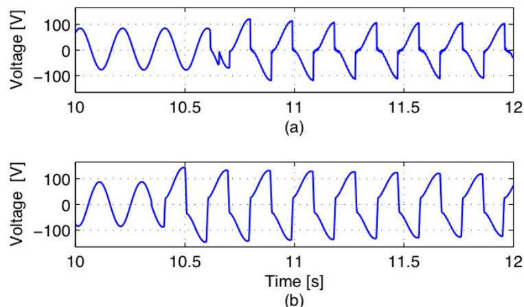
Figure 9. Detailed view of the electrical response after triggering the circuit breaker: (a) Using SSDS; (b) Using SSDI
