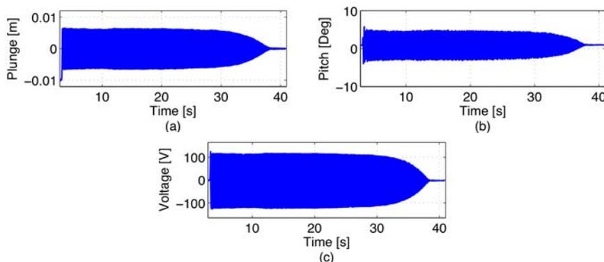
Figure 12. Plunge displacements (a), pitch displacement (b) and voltage (c) using SSDI, under 13.1 m/s airflow speed
