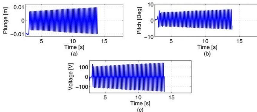
Figure 11. Plunge displacements (a), pitch displacement (b) and voltage (c) using SSDS, under 12.8 m/s airflow speed
