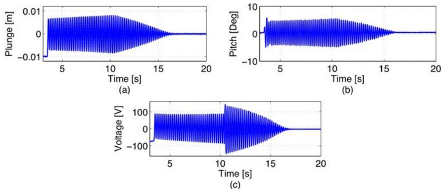
Figure 8. Time histories, using SSDI, of plunge displacements (a), pitch displacement (b) and voltage (c), at the linear flutter speed
