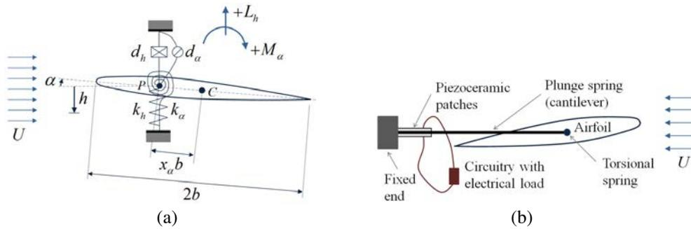
Figure 1. Aeroelastic typical section under airflow excitation (a) and Electroaeroelastic typical section with piezoelectric coupling on the plunge DOF and an external electrical load (b).
