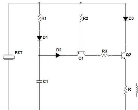
Figure 3. Circuit diagram of self-powered electronic breaker
