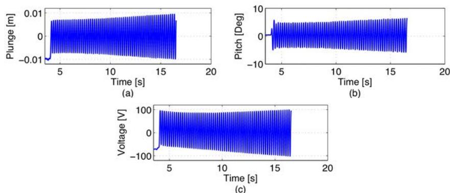
Figure 6. Time histories of plunge displacements (a), pitch displacement (b) and voltage (c), under airflow speed of 11,9 m/s
