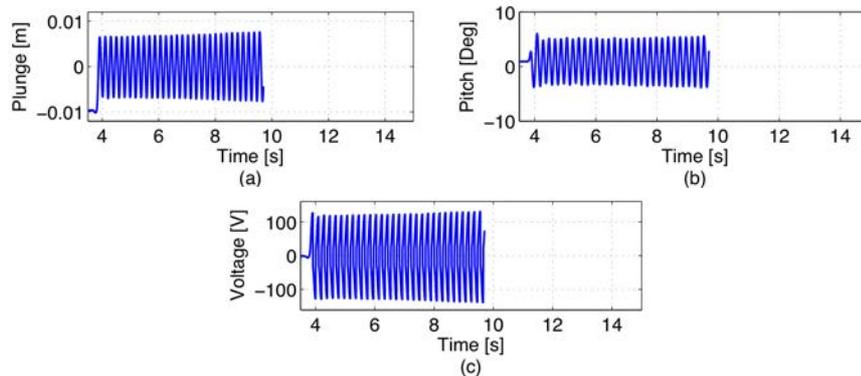
Figure 13. Plunge displacements (a), pitch displacement (b) and voltage (c) using SSDI, under 13.2 m/s airflow speed
