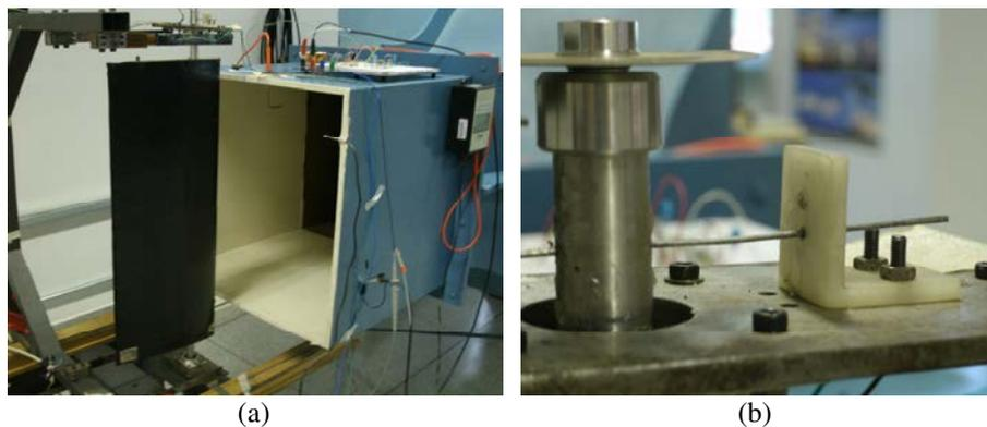
Figure 2. Experimental typical section (a) and detailed view of the pitch spring (b).
