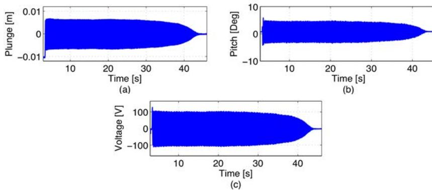
Figure 10. Plunge displacements (a), pitch displacement (b) and voltage (c) using SSDS, under 12.7 m/s airflow speed
