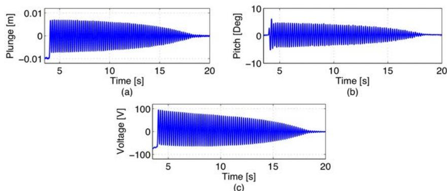
Figure 5. Time histories of plunge displacements (a), pitch displacement (b) and voltage (c), under airflow speed of 11,7 m/s
