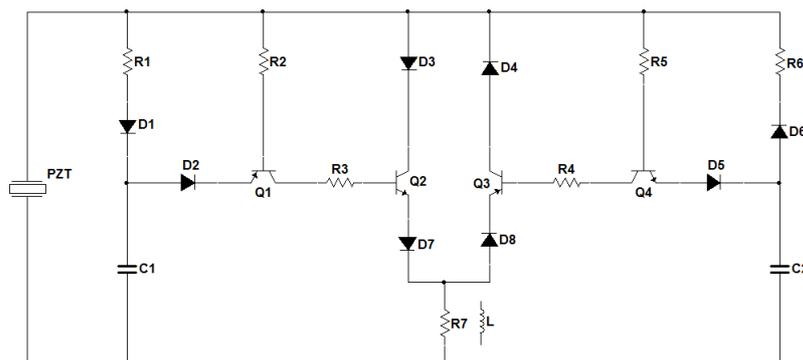
Figure 4. Circuit diagram of the self-powered full-wave electronic breaker
