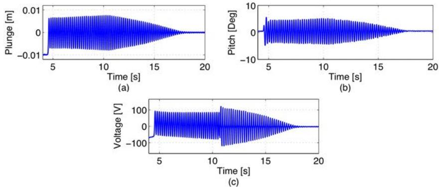
Figure 7. Time histories, using SSDS, of plunge displacements (a), pitch displacement (b) and voltage (c), at the linear flutter speed
