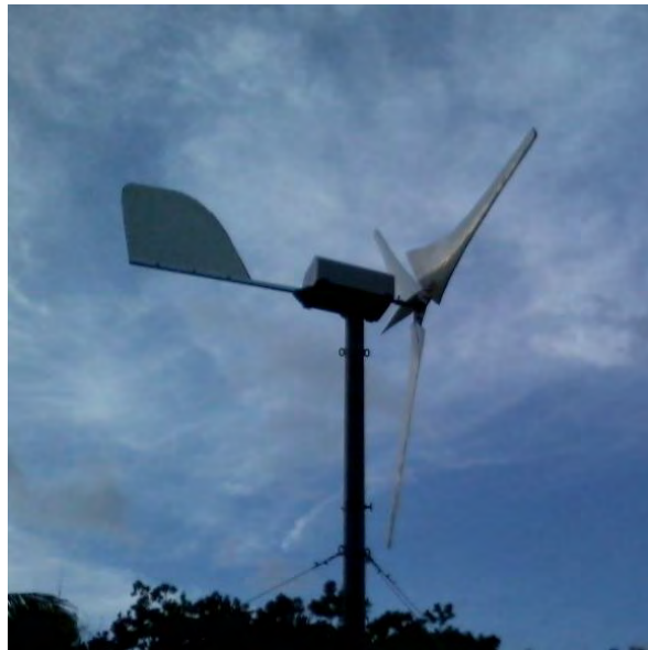
Figure 8. Guyed tower, rudder, nacelle and rotor
