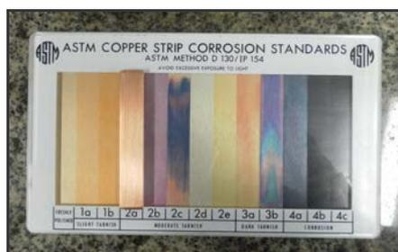
Figure 5: Comparison of the color of copper strip in ASTM standard after the test.
