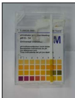
Figure 2. PH indicator paper and tape used for the determination of the pH of carnauba oil.
