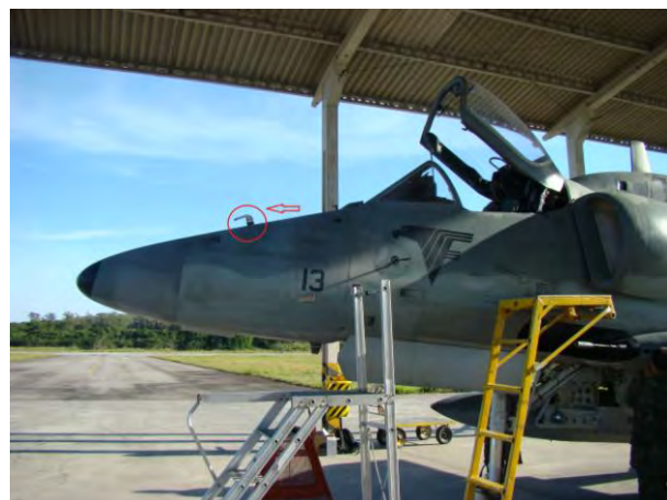
Figure 2. Pitot probe PH-510 mounted on the A4 Skyhawk aircraft of the Brazilian Navy, São Pedro d'Aldeia Naval Base.
