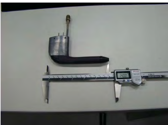
Figure 1. Pitot probe PH-510 used as the basis for the proposed thermal model.
