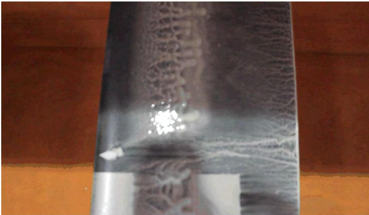
Figure 11. Image of NACA 0012 airfoil during flow-viz visualization ( $5^\circ$  angle of attack)
