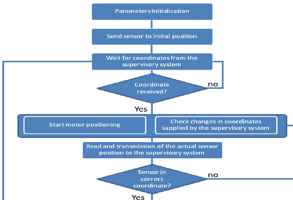
Figure 7. Positioning Algorithm Flowchart
