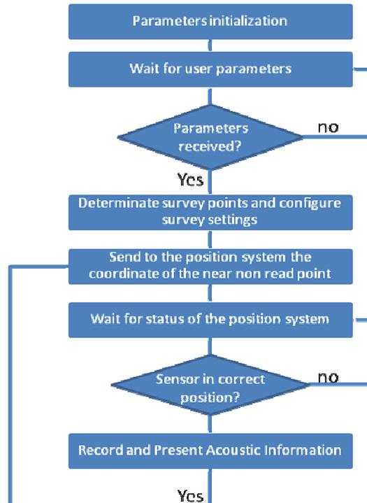
Figure 8. Supervisory System Algorithm
