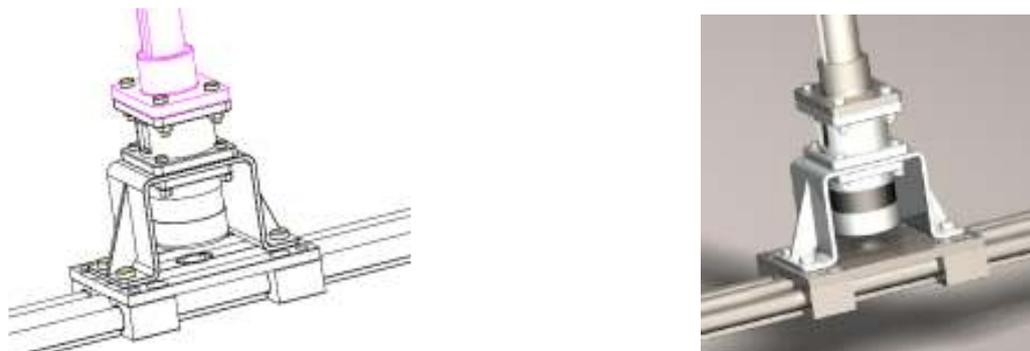
Figure 3. Link Between Horizontal and Vertical Displacement Systems
