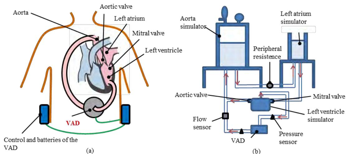
Figure 1. (a) Schematic of a VAD implanted inside the body and (b) schematic of a mock circulatory loop
