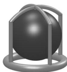
Figure 3. Caged-ball valve.
