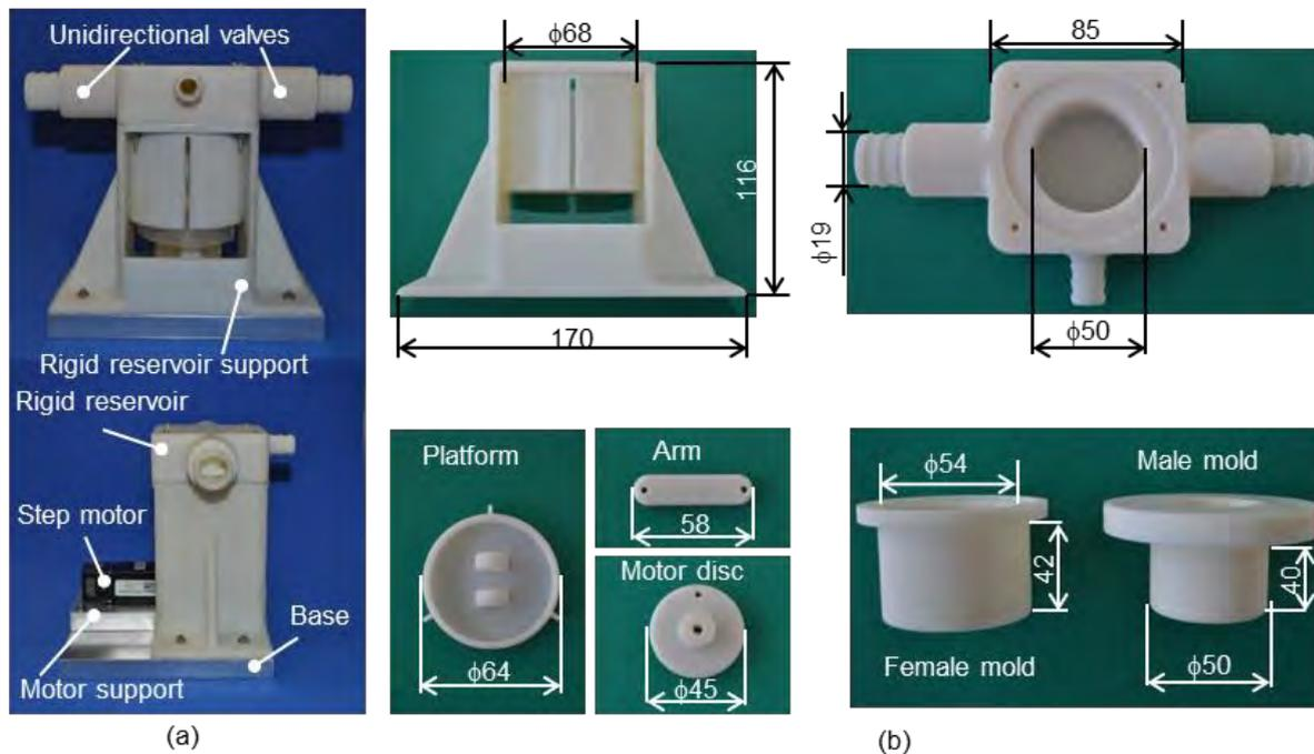
Figure 4. (a) Pulsatile pump to simulate the left ventricle and (b) printed components of the pump
