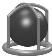
Figure 3. Caged-ball valve.
