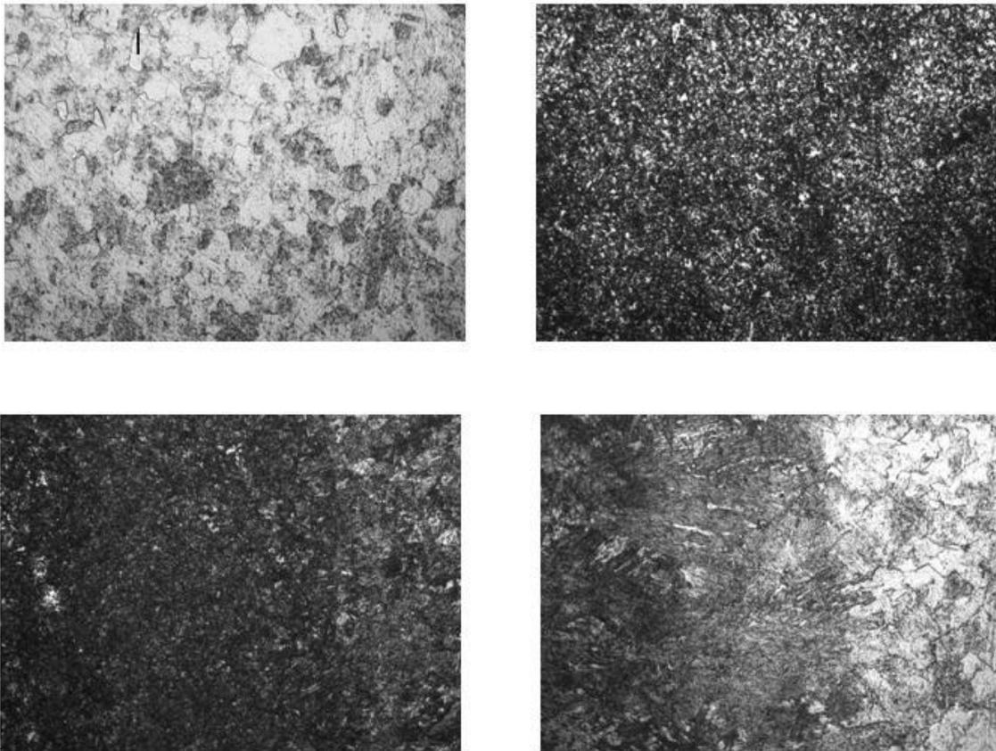
**Figure 7:** Different regions of the sample 3 (shallow section). Attack: 2% Nital. 50x magnification.
