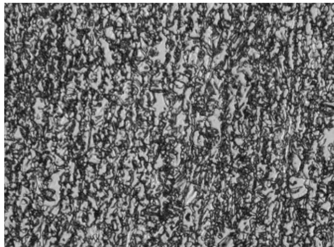
**Figure 4:** Microstructure - TRIP 800 steel. etching: Nital 2%. Magnification: 500x.
