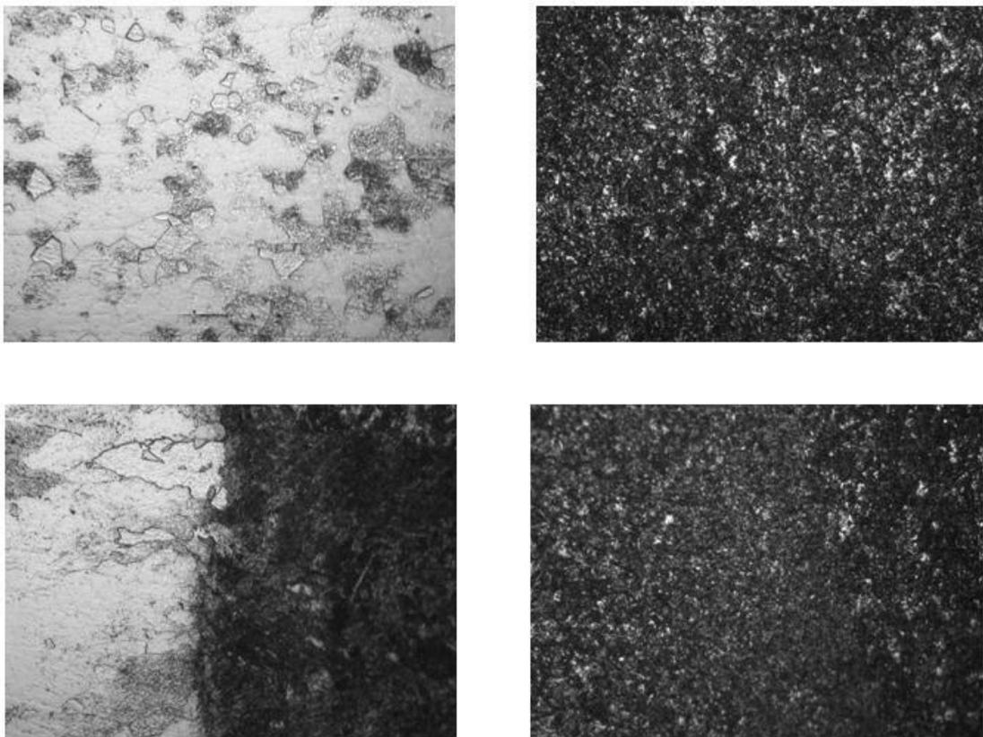
**Figure 8:** Different regions of the sample 4 (shallow section). Attack: 2% Nital. 200x magnification.
