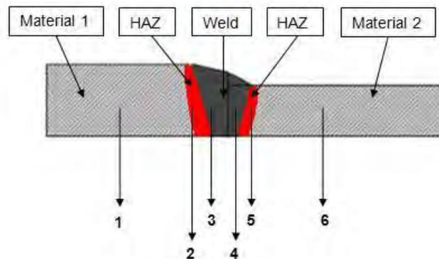
Figure 9: Areas of testing microhardness.
