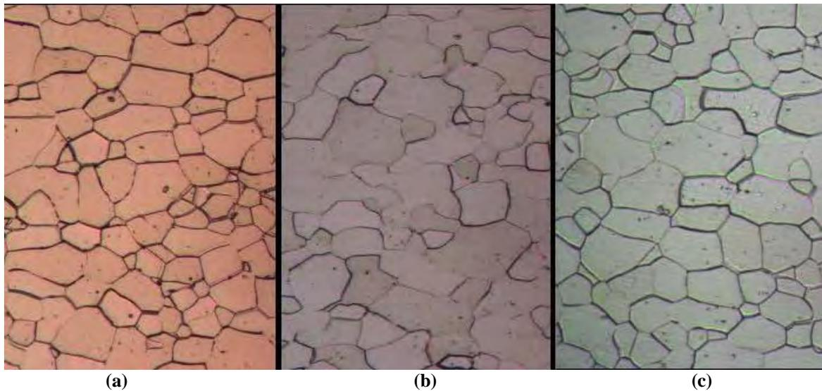
**Figure 3:** (a) Low-carbon longitudinal, magnification 500x. (b) Interstitial-free longitudinal, magnification 500x. (c) bake-hardening longitudinal, magnification 500x.
