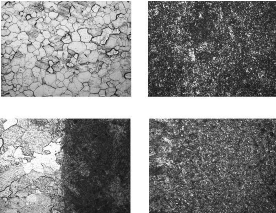
**Figure 6:** Different regions of the sample 2 (shallow section). Attack: 2% Nital. 200x magnification.
