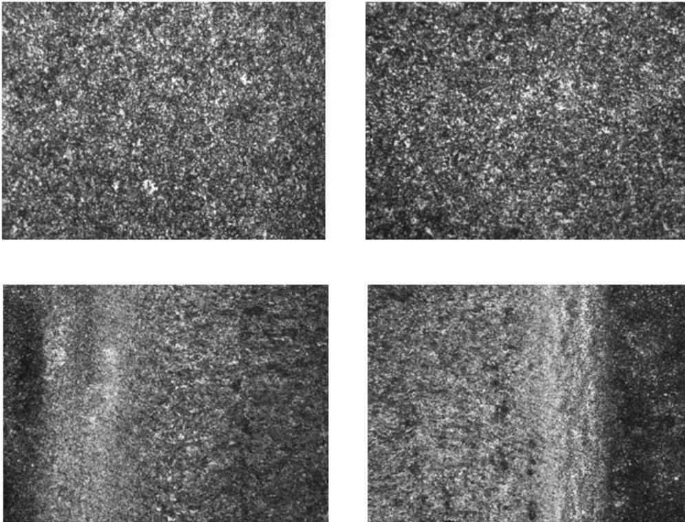
**Figure 5:** Different regions of the sample 1 (shallow section). Attack: 2% Nital. 50x magnification.
