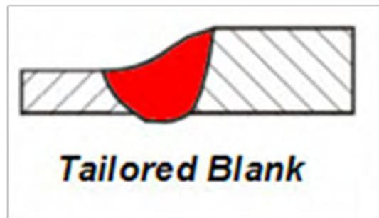
Figure 1- Junction of two blanks by laser weld.
