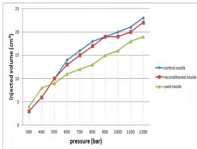
Figure 11: Injection volume of nozzles
