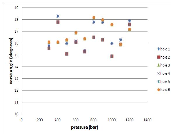
Figure 19: Cone angle (reconditioned nozzle)
