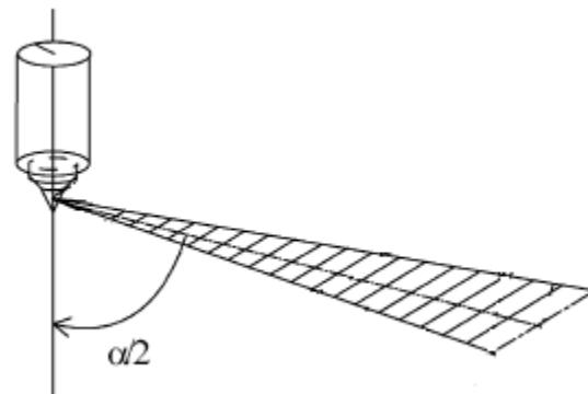
**Figure 6: Injection angle**
