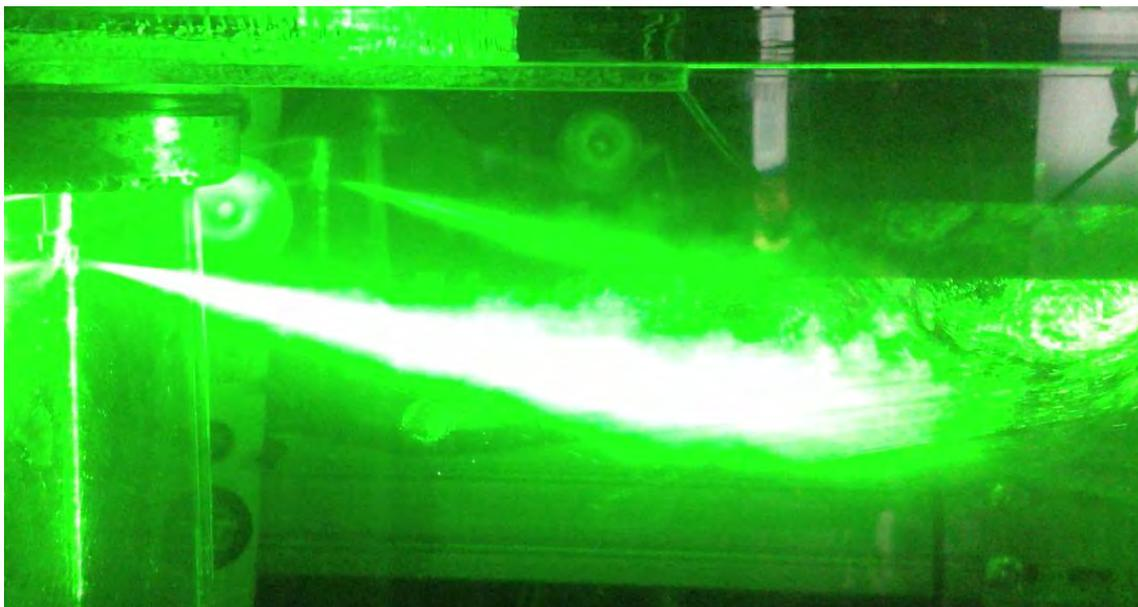
**Figure 9: Atomized jet fully developed**
