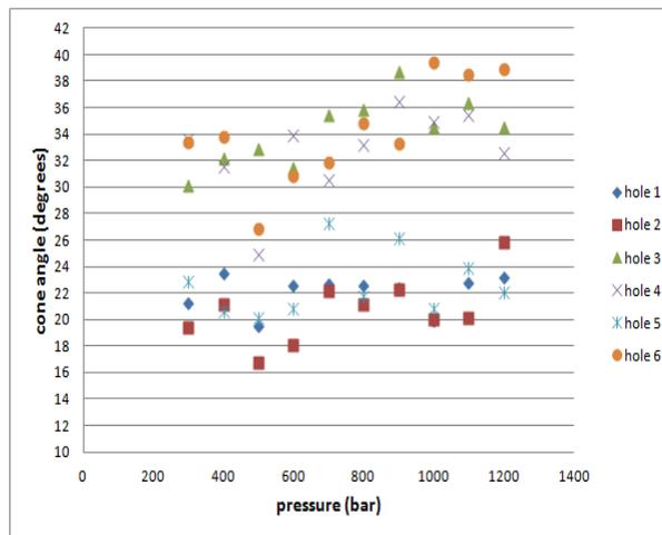
Figure 20: Cone angle (used nozzle)
