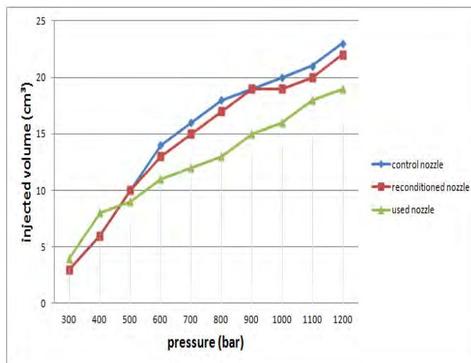
**Figure 11: Injection volume of nozzles**
