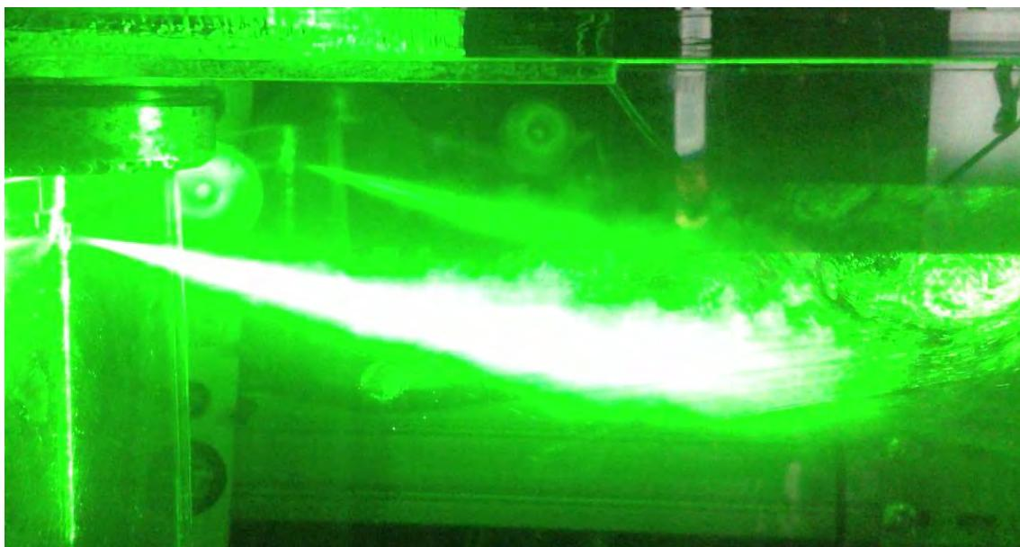
**Figure 9: Atomized jet fully developed**
