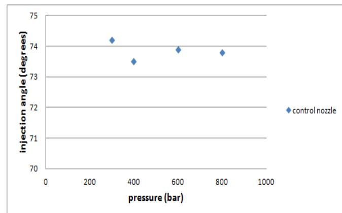
**Figure 15: Injection angle x injection pressure (control nozzle)**
