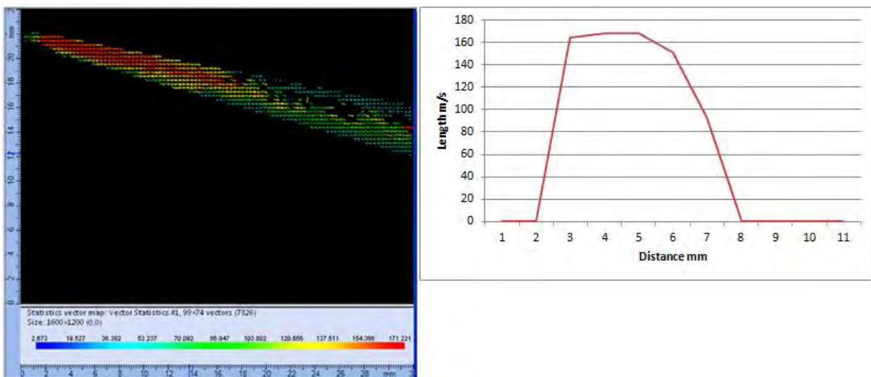
Figure 22: Velocity field and velocity profile of refurbished nozzle injector
