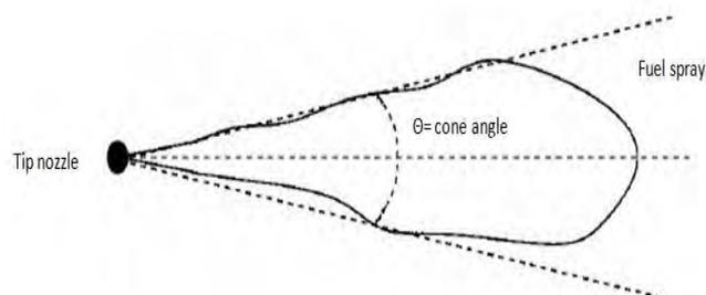
**Figure 7: Cone angle of atomized jet.**
