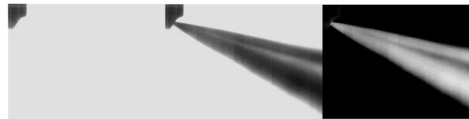
**Figure 12: Frames of atomized jet normal to the CCD**
