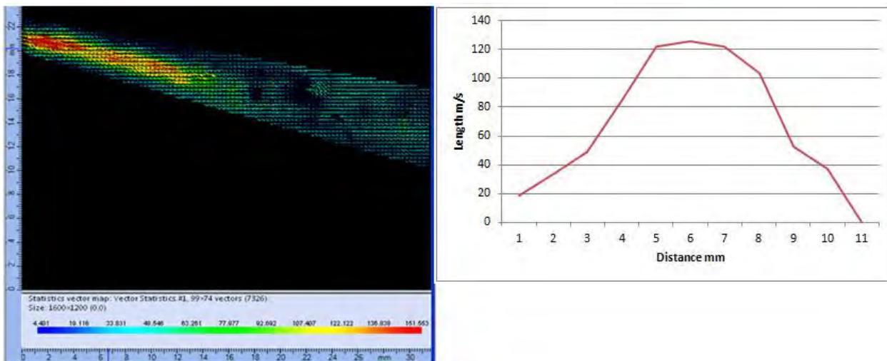
Figure 22: Velocity field and velocity profile of used nozzle injector
