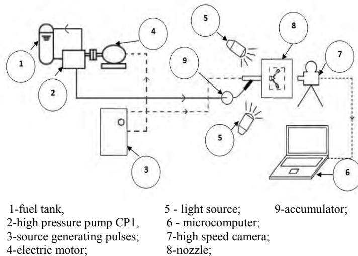
**Figure 3: Schematic of experimental setup.2**
