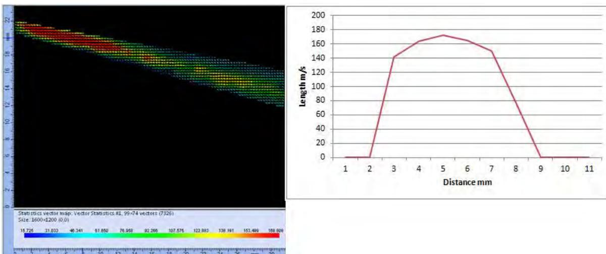
Figure 21: Velocity field and velocity profile of new nozzle injector
