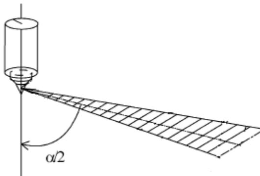
**Figure 6: Injection angle**
