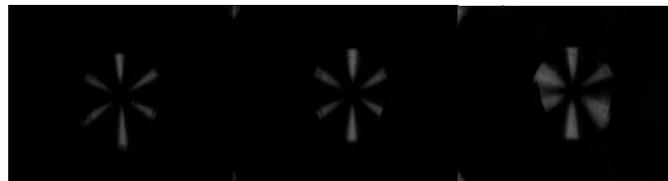
Figure 17: Sprays of control, reconditioned and used nozzle, respectively
