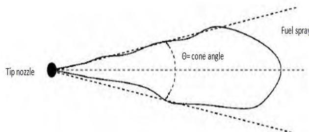
**Figure 7: Cone angle of atomized jet.**
