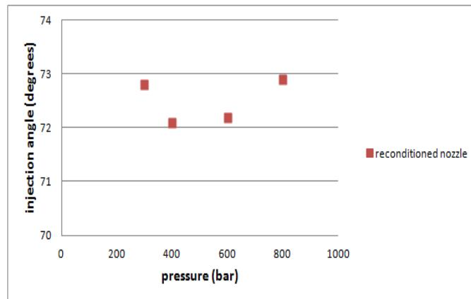
**Figure 16: Injection angle x injection pressure (reconditioned nozzle)**
