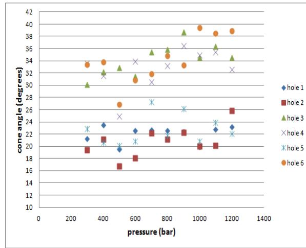
Figure 20: Cone angle (used nozzle)
