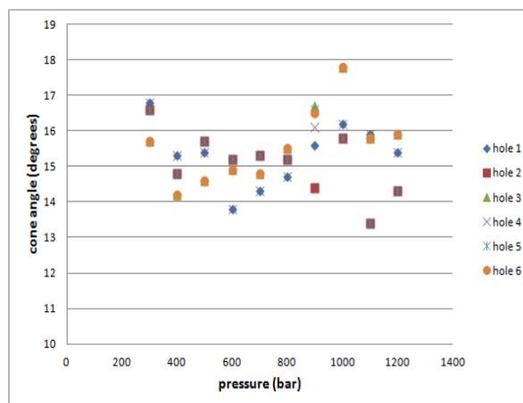
Figure 18: Cone angle (control nozzle)
