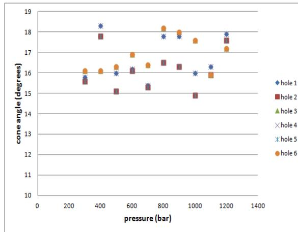
Figure 19: Cone angle (reconditioned nozzle)
