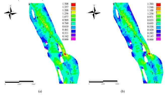
Figure 8. Velocity Magnitude Isosurface (m/s) of June (a) and July (b)
