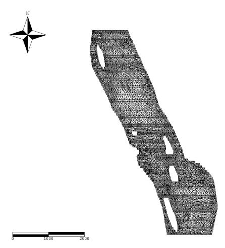
Figure 4. Finite Elements Mesh for the Hydrodynamic Model
