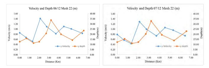
Figure 11. Velocity and depth profile graphics of June and July
