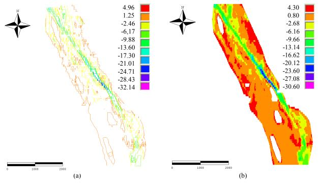
Figure 3. Raw (a) and Interpolated (b) Terrain Elevation Model (m)
