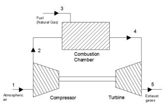
Figure 1 - Schematic representation of the gas turbine
