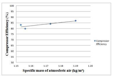
Figure 4 - Compressor efficiency in relation to specific mass of atmospheric air
