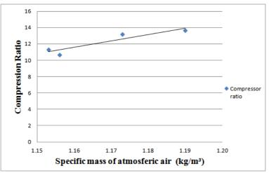
Figure 6 - Compression ratio in relation specific mass of atmospheric air
