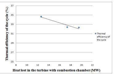
Figure 10 - Thermal efficiency of the cycle in relation heat lost in the turbine with combustion chamber
