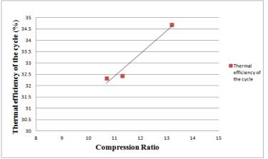
Figure 1 - Thermal efficiency of the cycle in relation compression ratio
