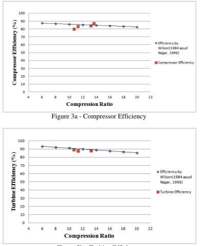
Figure 3b - Turbine Efficiency
