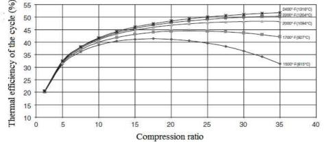
Figure 2 - The thermal efficiency of the cycle relative to pressure ratio based on compressor efficiency of 87% (Source: Boyce, 2006)
