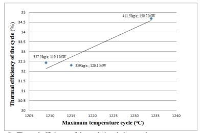
Figure 8 - Thermal efficiency of the cycle in relation maximum temperature cycle
