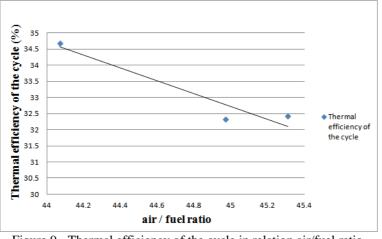
Figure 9 - Thermal efficiency of the cycle in relation air/fuel ratio
