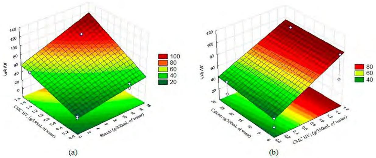
Figure 3. Response surfaces for AV, setting: (a) concentration of calcite at 12.5g/350mL of water and (b) concentration of starch at 12g/350mL of water.
