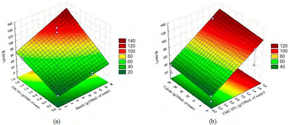
Figure 5. Response surfaces for YL, setting: (a) concentration of calcite at 12.5g/350mL of water and (b) concentration of starch at 12g/350mL of water.
