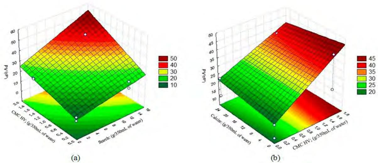
Figure 4. Response surfaces for PV, setting: (a) concentration of calcite at 12.5g/350mL of water and (b) concentration of starch at 12g/350mL of water.
