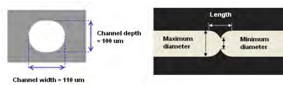
Figure 4. Cross section of the channels and dimensions of the throat
