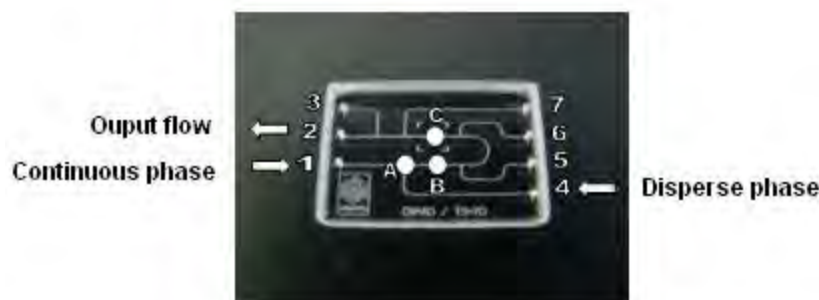
Figure 5. Microcapillary used, showing the input and output flow, the region of oil drop formation and the regions evaluated in the flow
