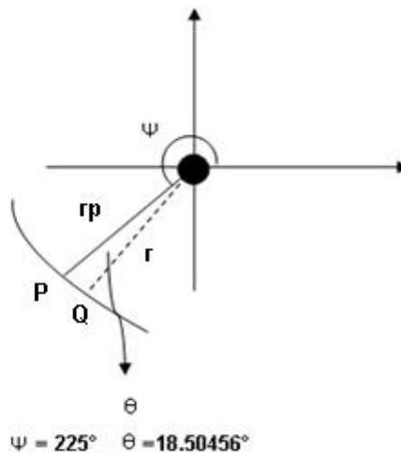
Figure 6. Geometry of the system for the case of maximum variation of energy for  $\psi=225^\circ$  and  $\delta V=0.5$ .
