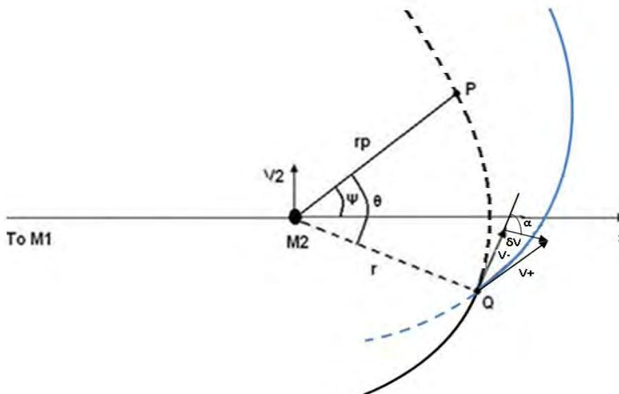
Figure 1. Geometry of the Swing-By with the application of the impulse out of the periapsis.
