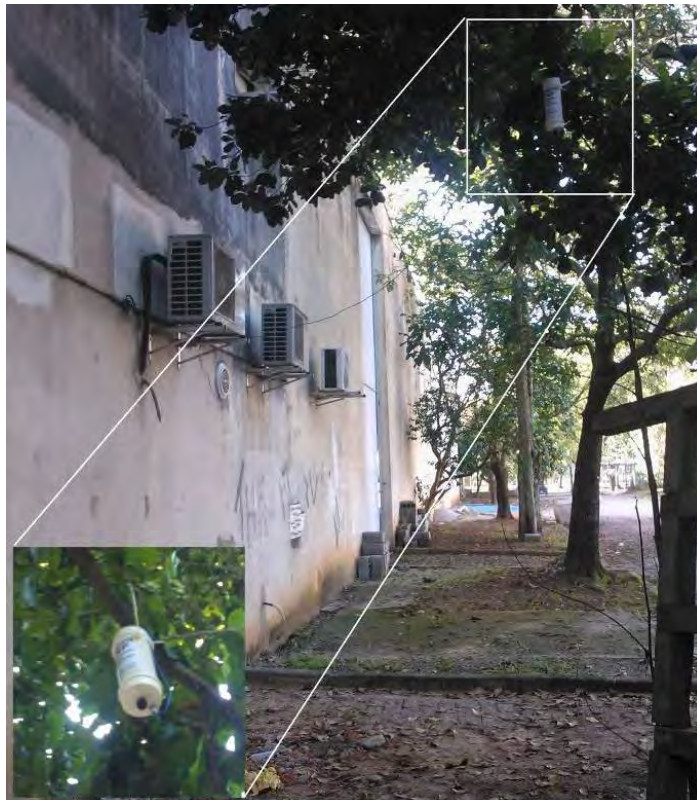
Figure 3. AVAMS prototype with Raspberry Pi and POE installed in the Poli/USP campus
