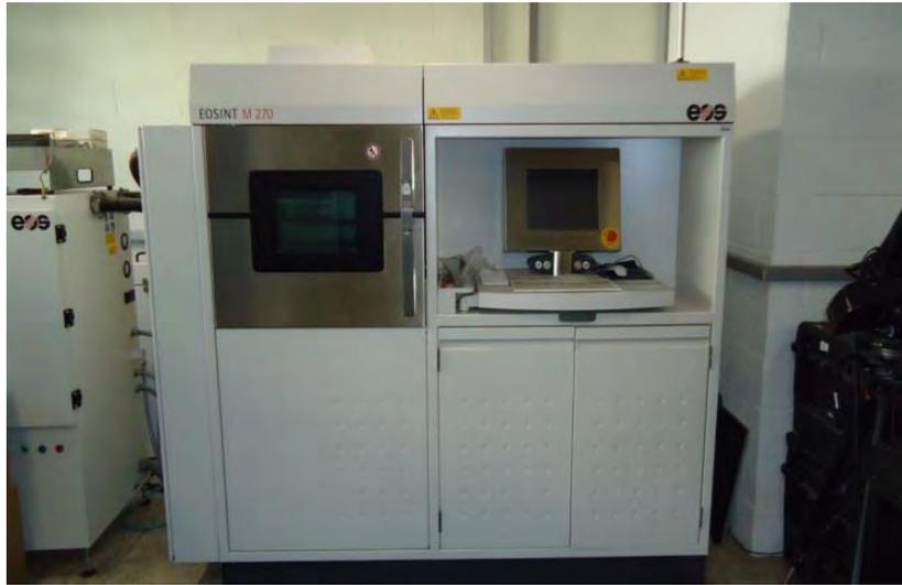
Fig. 2 - Rapid Prototyping Machine (EOSINT M270).
