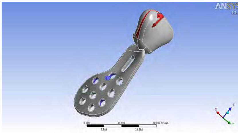
Fig. 6 - Simulating with three fixing screws.
