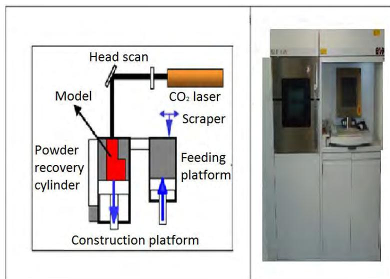
Fig. 1 - Schematic diagram of the DMLS process and EOSINT prototyping machine.
