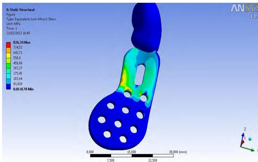
Fig. 7 - Finite element analysis of the Von-Mises stresses for three screws.
