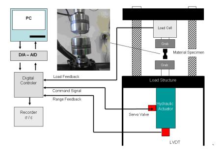
Figure 14. Uniaxial fatigue testing equipment
