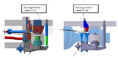
Figure 3. Vehicle lateral kinematics from CAD kinematic analysis
