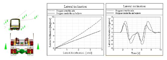
Figure 4. Vehicle lateral behavior from CAE multibody analysis
