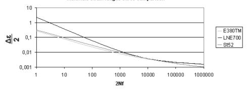
Figure 9. Experimental strain-life curves obtained for the materials
