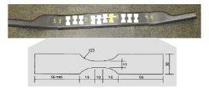
Figure 8. Geometry and dimensions [mm] of the specimens taken from manufactured parts.
