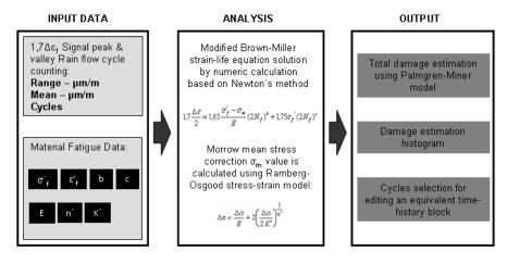
Figure 11. Program algorithm for VBA implementation
