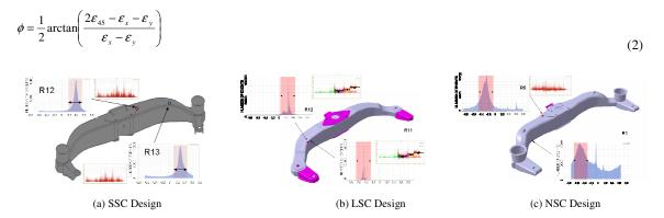
Figure 10. Highest measured RMS strain values positions and signal proportionality
