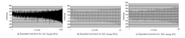
Figure 13. Equivalent load blocks for the three designs of fatigue spectra
