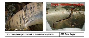
Figure 12. Fatigue failure event during the standard durability track testing program>
