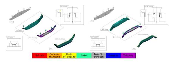
Figure 7. FEM stamping results for the four stages assumed in the production concept
