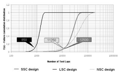
Figure 15. Weibull curves showing the expected B10 life for each design.
