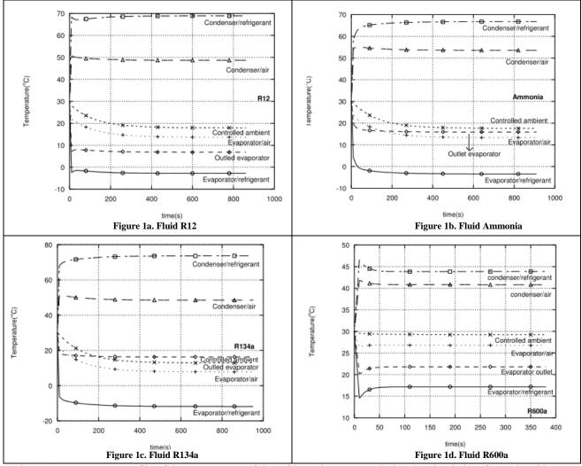
Figure 1. Temperature profile of the components of the refrigeration system, during the simulation, for each refrigerant examined.
