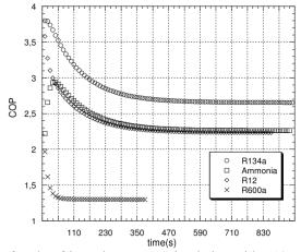
Figure 2. COP of each refrigeration system simulation with R12, R134a, Ammonia and R600a.
