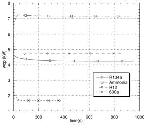
Figure 4 show that the simulated system with R600a has consumed the least amount of energy, because it required approximately 2.6 kW compressor power. However, the system simulated with R600a didn't reduce the temperature of the cooling chamber, as shown in Figure 1d. The systems with R12 and R134a have similar energy cost, because the compressor power was between 4 and 5 kW.
