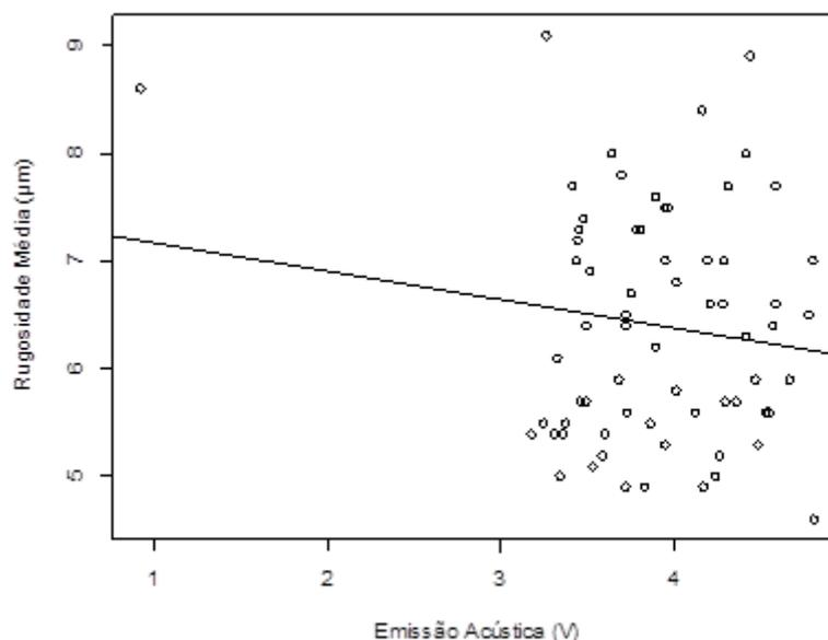
Figure 5 - Graph of linear regression for the average roughness (Ra) as a function of acoustic emission in the sanding of *Corymbia citriodora*.
