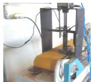
Figure 2 (a) Surface Roughness Tester used to determine the roughness of the sanded surfaces
