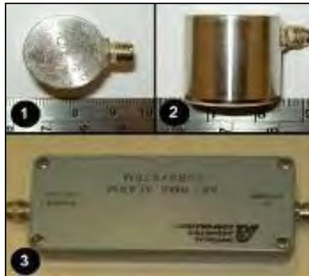
Figure 3 - Module Acoustic emission (1) sensor (2) and amplifier (3).
