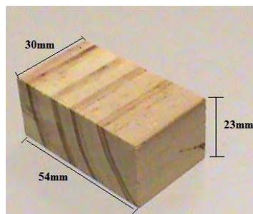
Figure 1 - Dimensions of the specimens.
