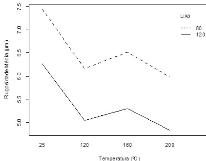
Figure 4 - Graph of the roughness average (Ra) as a function of temperature for each abrasive particle in the samples heat treated and control samples (25 ° C), in the sanding of *Corymbia citriodora*.
