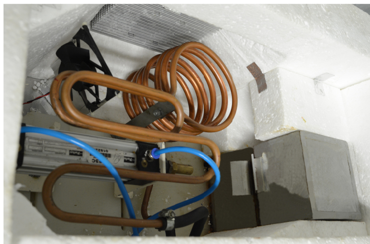
Figure 1. Direct measurement of the adiabatic temperature change apparatus.
