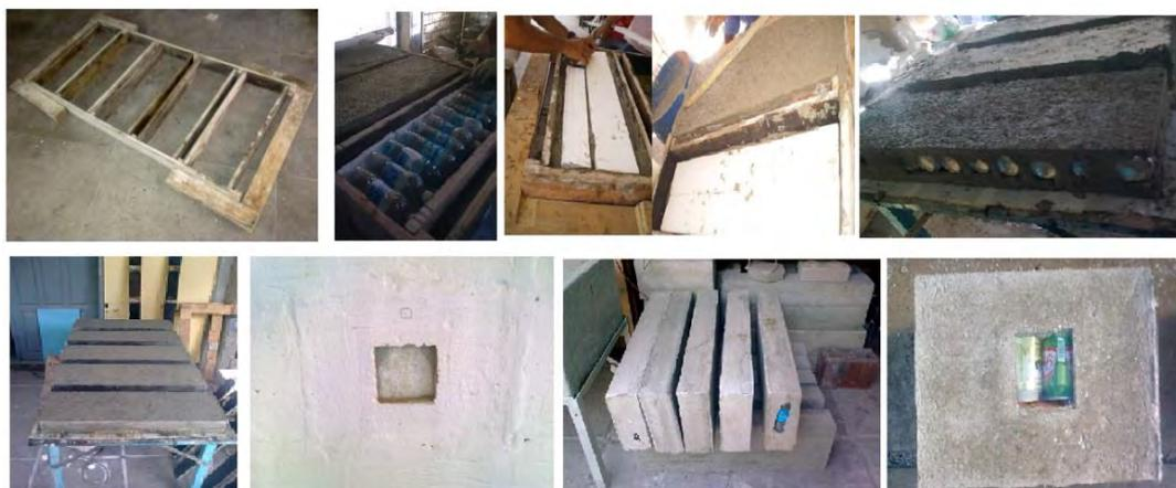
Figure. 2. Manufacturing steps of blocks with three fillings used.
