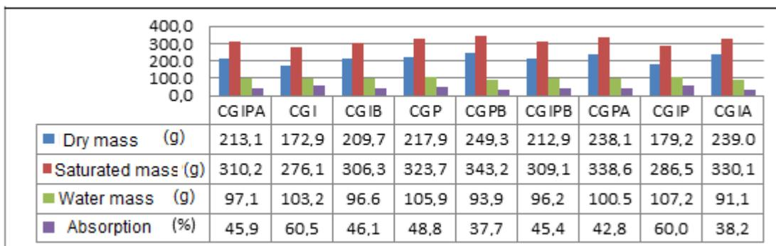
Figure 5. Behavior of parameters in water absorption test.
